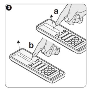
Touching and sliding activate different commands, based on the automation used and the programming carried out. The slider function on the remote control send a RF signal like to press a button (e.g. Up, down, stop) and set level in the climatic sensor (not in the scope of this certification). The transmissions signal is same of a remote command by pressing a buttons.
