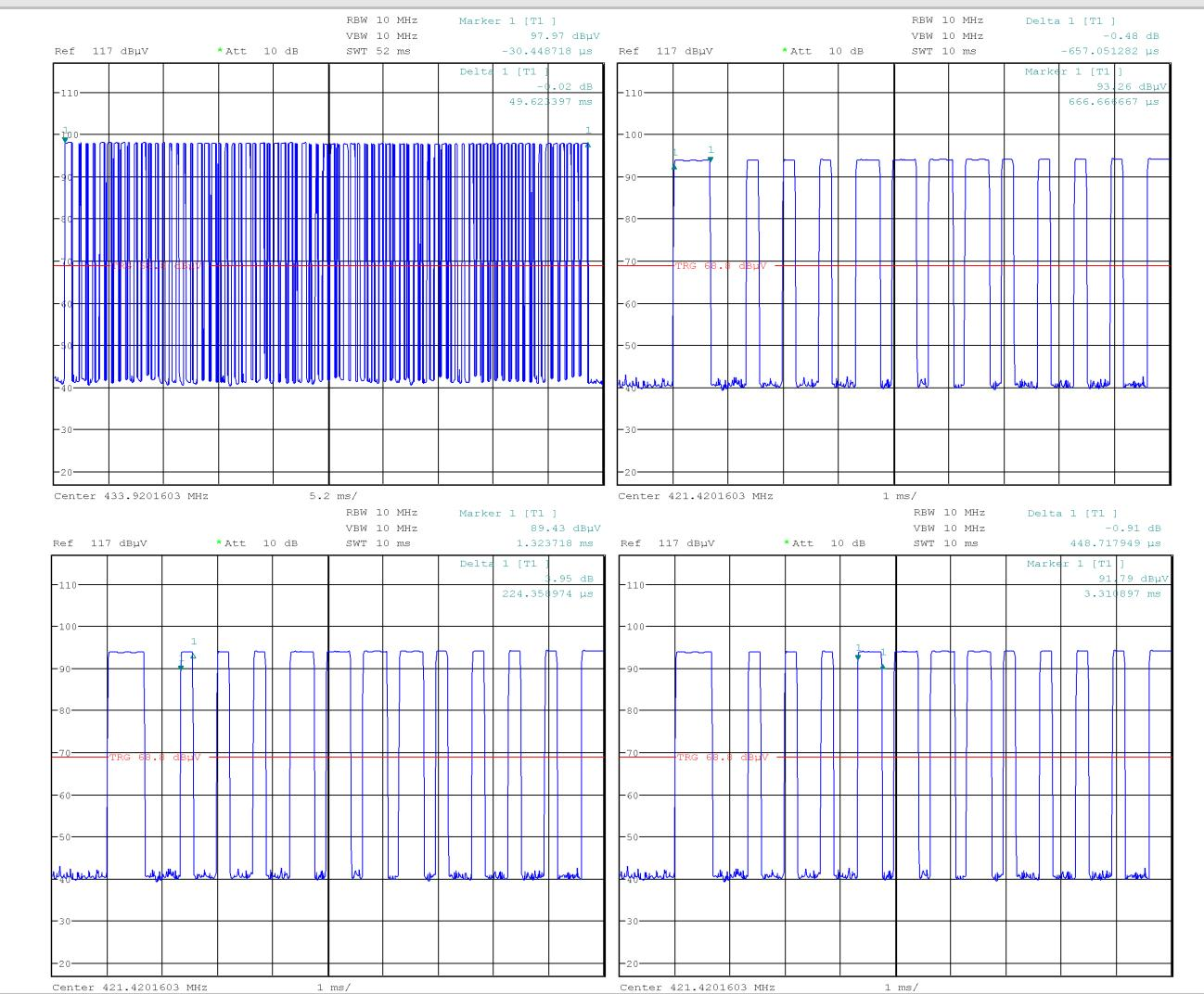
After activation of transmission the equipment send 5 codes and then ceases the transmission.
