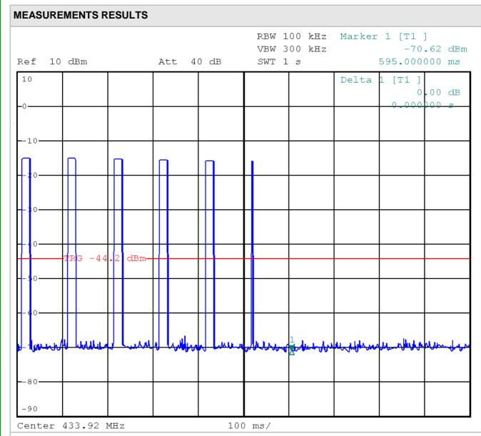
After activation of transmission the equipment send 6 pulses train and then ceases the transmission.
