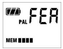
Wait for 5s, or press Mode button 2 times or press Power button 2 times, it will save the PAL system
