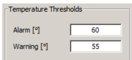
4. Select the Temperature THRESHOLD level and the Warning level.
