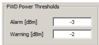
3. Select the FWD power THRESHOLD level and the Warning level.
