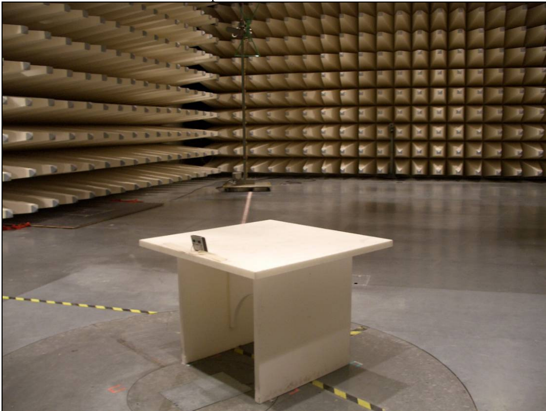
Photo 8: setup of radiated emission of the EUT B
