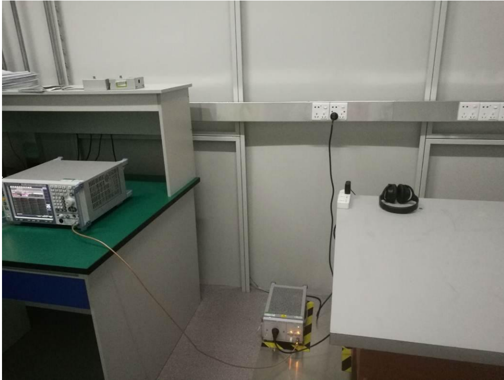
FCC RADIATED EMISSION TEST SETUP
