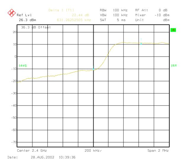
This graph indicates compliance on the lower band edge. The center of the lowest channel is 2.4012 GHz.
