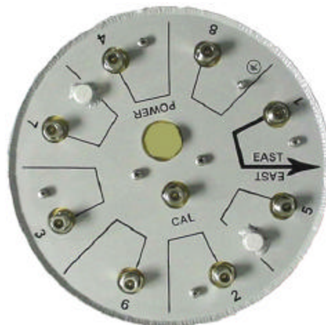
Figure 30: Bottom of an Omni Antenna Showing Correct Orientation
