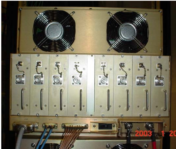
Figure 37: Split Chassis RF/PA Shelf Rear View
