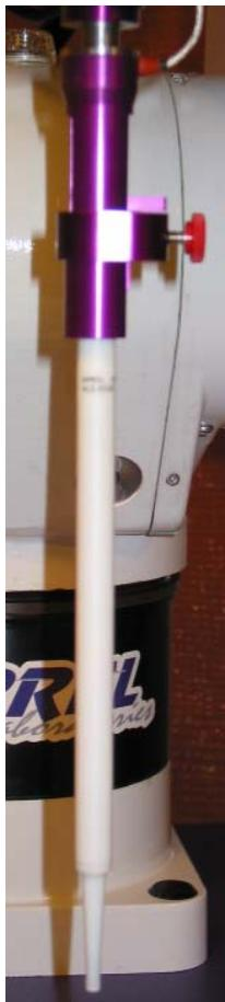
The Aprel E-Field probe is evaluated to establish the diode compression point.
