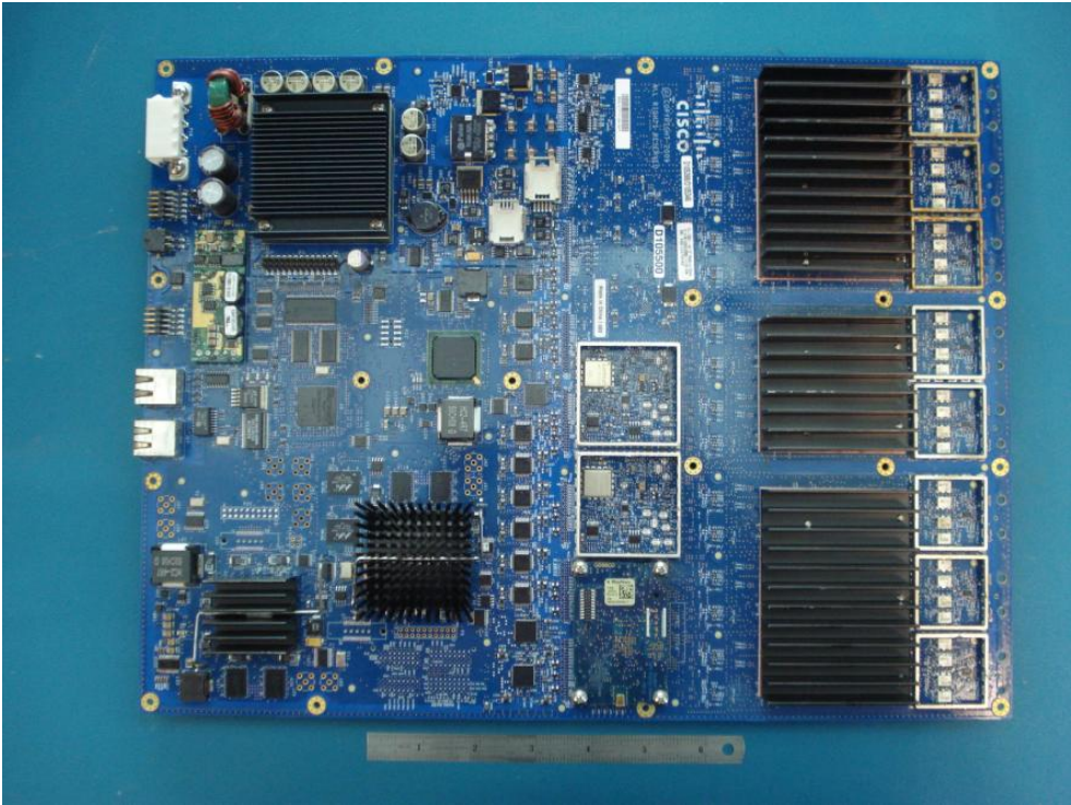
Low Power RF Board (note ruler is 6-inch)
