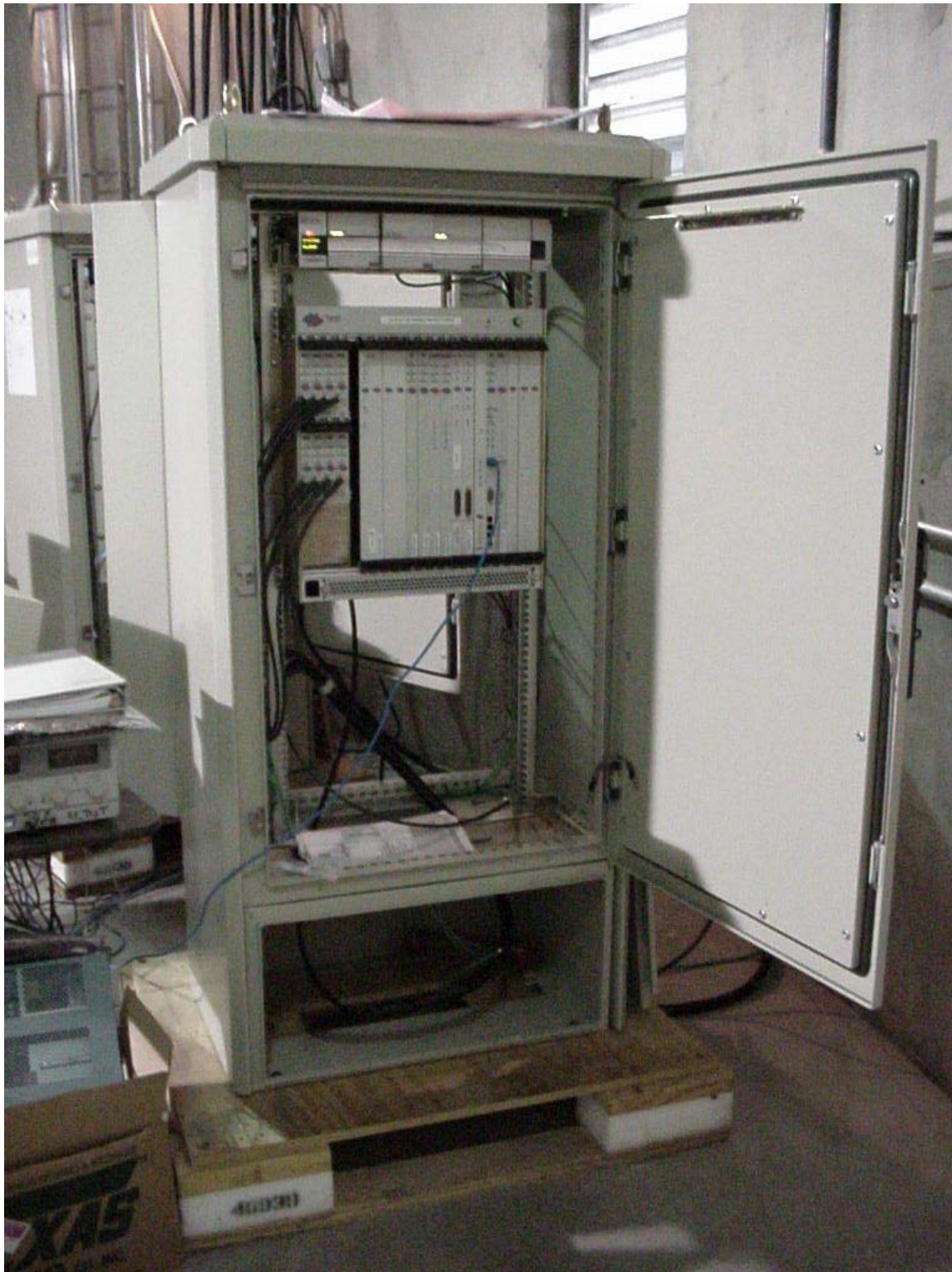
Figure C7: TTA Digital Chassis (Front)
