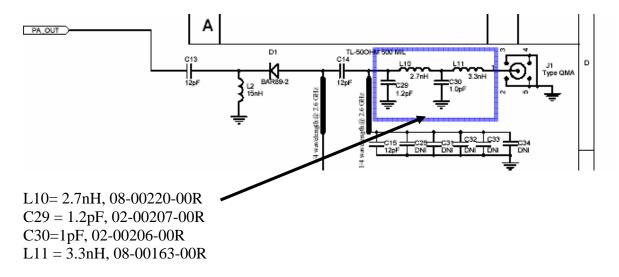
Also SUBBED in a Peak Devices part: 29-00046-00R for 2.3 TTA module 29-00045-00R for 2.5 and 2.6 TTA module
