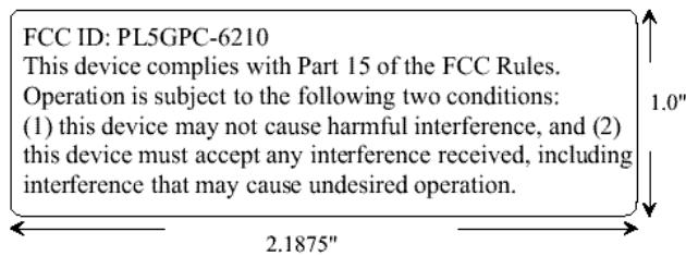
**Specifications:** Text is black or white in color and is left justified. Labels are silk-screened and shall be "permanently affixed" at a conspicuous location on the EUT.
