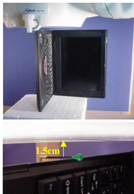
Body SAR Test Setup 1 1.5cm Antenna Separation Distance Antenna Parallel to Planar Phantom
