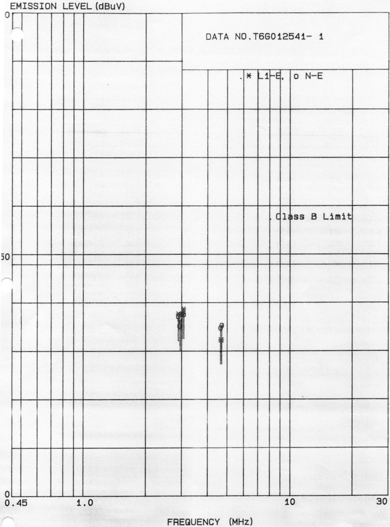
Figure 6.1-1 RFI Voltage Measurement Results
