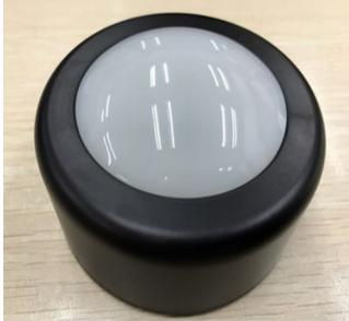
**Me First** uses 2.4GHz technology. The effective distance is **30 meters minimum**, and should be more with current technology. One master FCU (Facilitator's Control Unit) should be able to **connect with stability to 36 answer PADs** (Personal Answer Dome). The selling unit is 1 master with 12 answer pads and 1 pc USB cable (1.3m) in a box.
