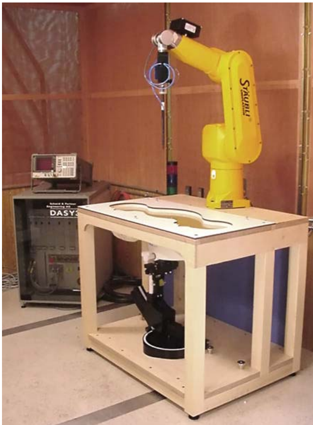
DASY3 SAR Measurement System with SAM phantom
