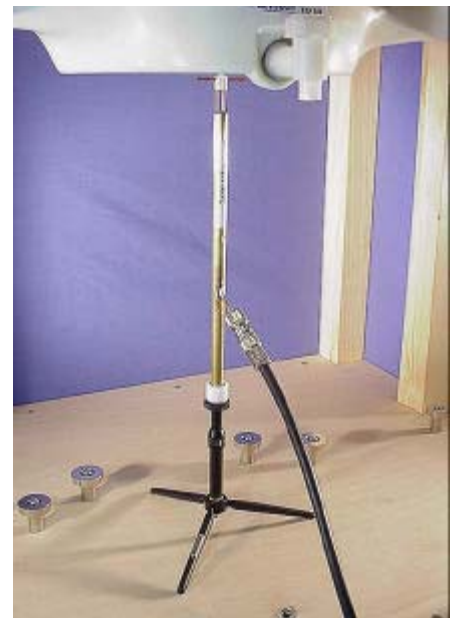
2450MHz Dipole Validation Setup
