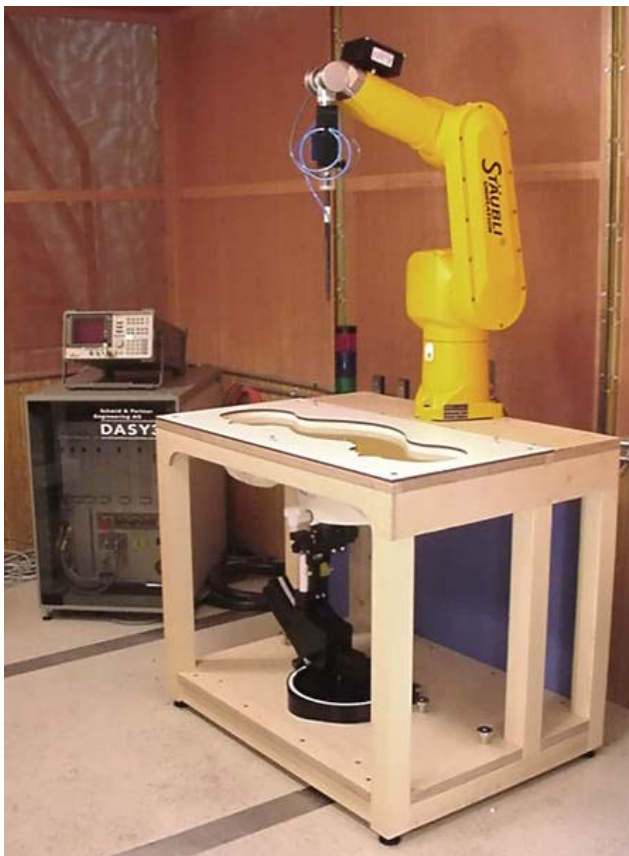
DASY3 SAR Measurement System with SAM phantom
