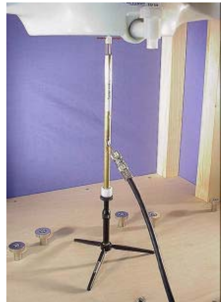
2450MHz Dipole Validation Setup
