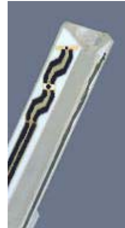
ET3DV6 E-Field Probe
