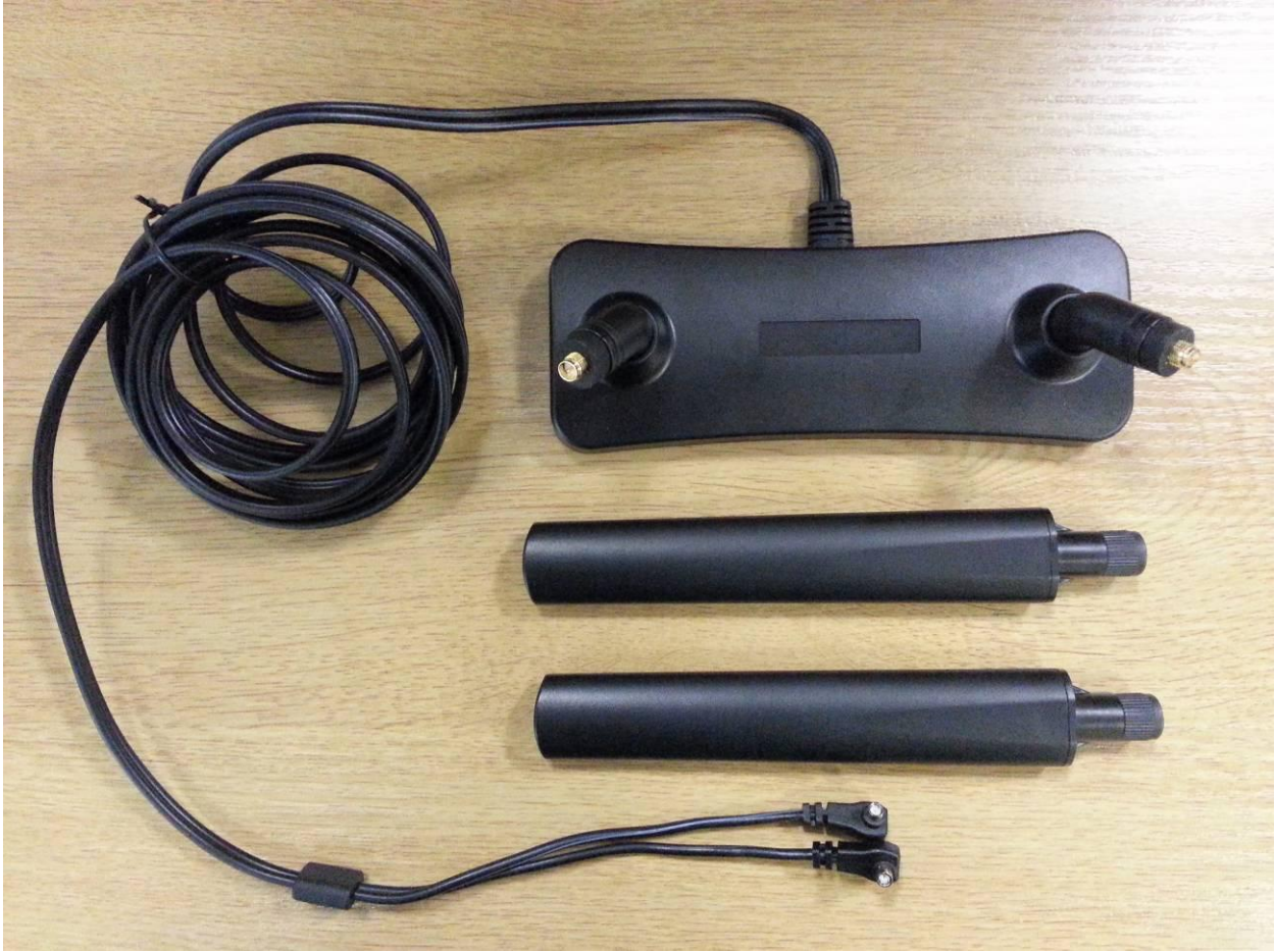
Figure 2: Remote Antenna Disassembled
