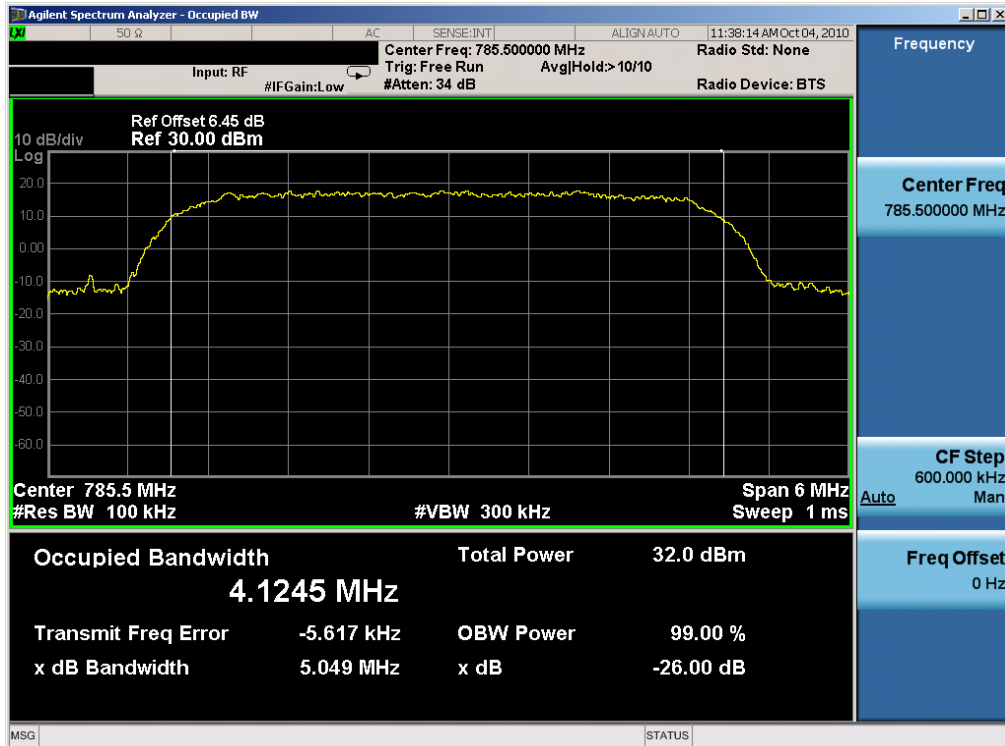
Plot 7-35. Occupied Bandwidth Plot (16QAM, Tx=785.5MHz)
