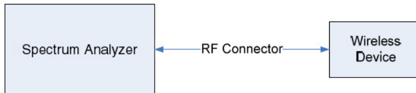
Figure 6-1. Conducted Output Power Test Setup Diagram
