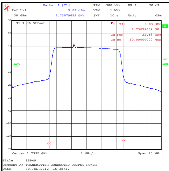
16QAM / 50 Resource Blocks
