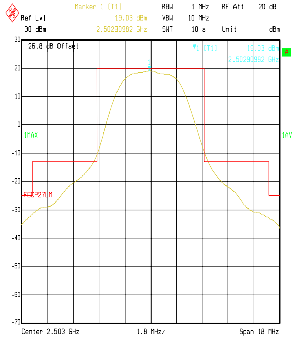
Title: IPWireless EUT:FD, FCC P27 Channel Edge Conducted Emissions Comment A: 47147JD02 Bottom Channel Low Chip Rate Date: 08.APR.2005 13:48:48
