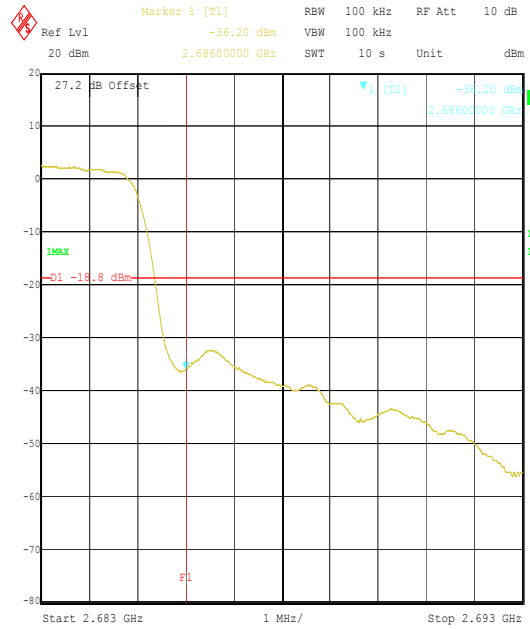
Title: IPWireless EUT: FD, FCC P15/21/74, Radiated BandEdge Comment A: 45219JD01 Top Channel 3.84 Mcps. Date: 4.FEB.2004 14:49:40
