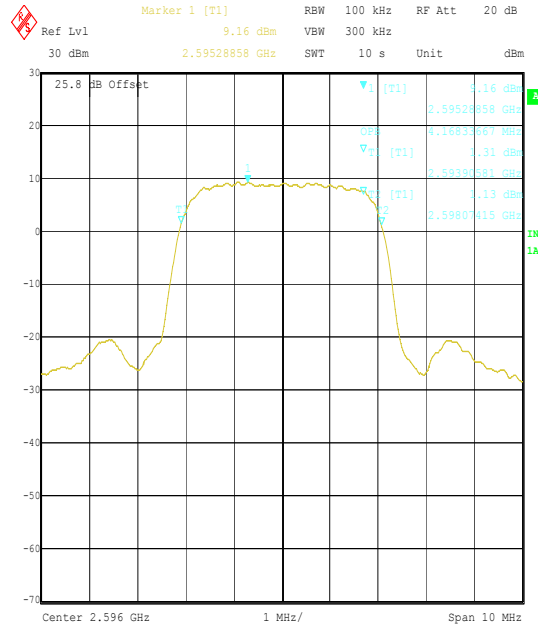
Title: IPWireless EUT: FD, FCC P15/21/74, Occupied Bandwidth Comment A: 45219JD01 Middle Channel 3.84 Mcps. Date: 5.FEB.2004 12:12:08
