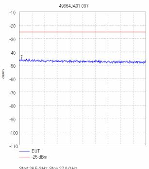
Start 26.5 GHz; Stop 27.0 GHz Ref -10 dBm; Ref Offset 43.0 dB; 10 dB/div RBW 1.0 MHz; VBW 1.0 MHz; Att 0 dB; Swp 50.0 mS Peak 26.509167 GHz, -44.5 dBm Display Line: -25 dBm; ; Limit Test Passed Tested by jxh 30/08/2007 14:13:11
