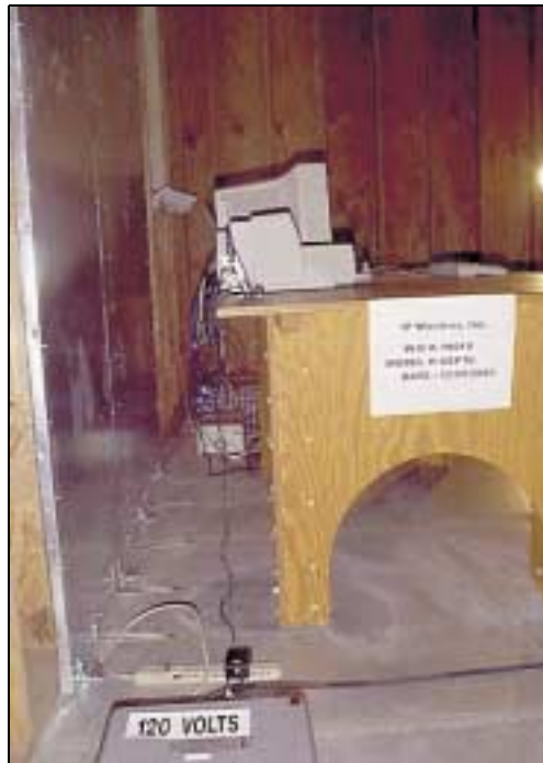
Mains Conducted Emissions Test Setup - Side View
