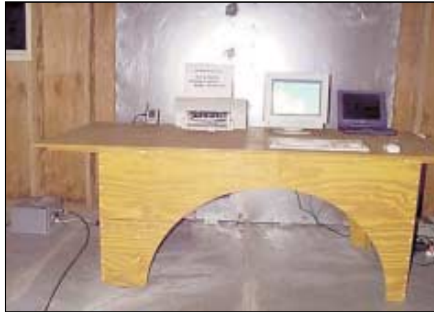
Mains Conducted Emissions Test Setup - Front View
