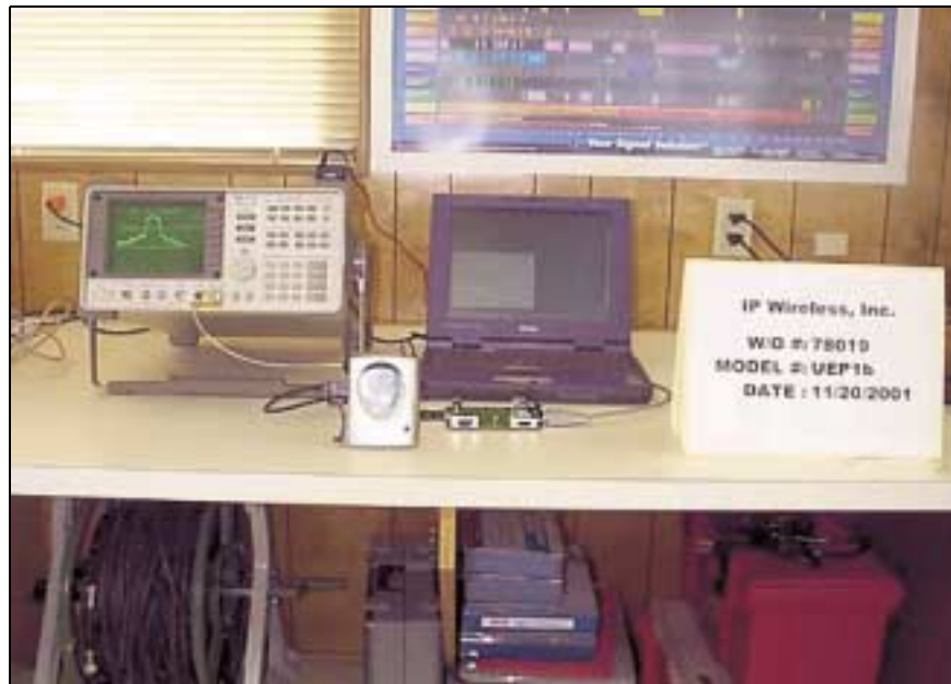
RF Output and Occupied Bandwidth Test Setup
