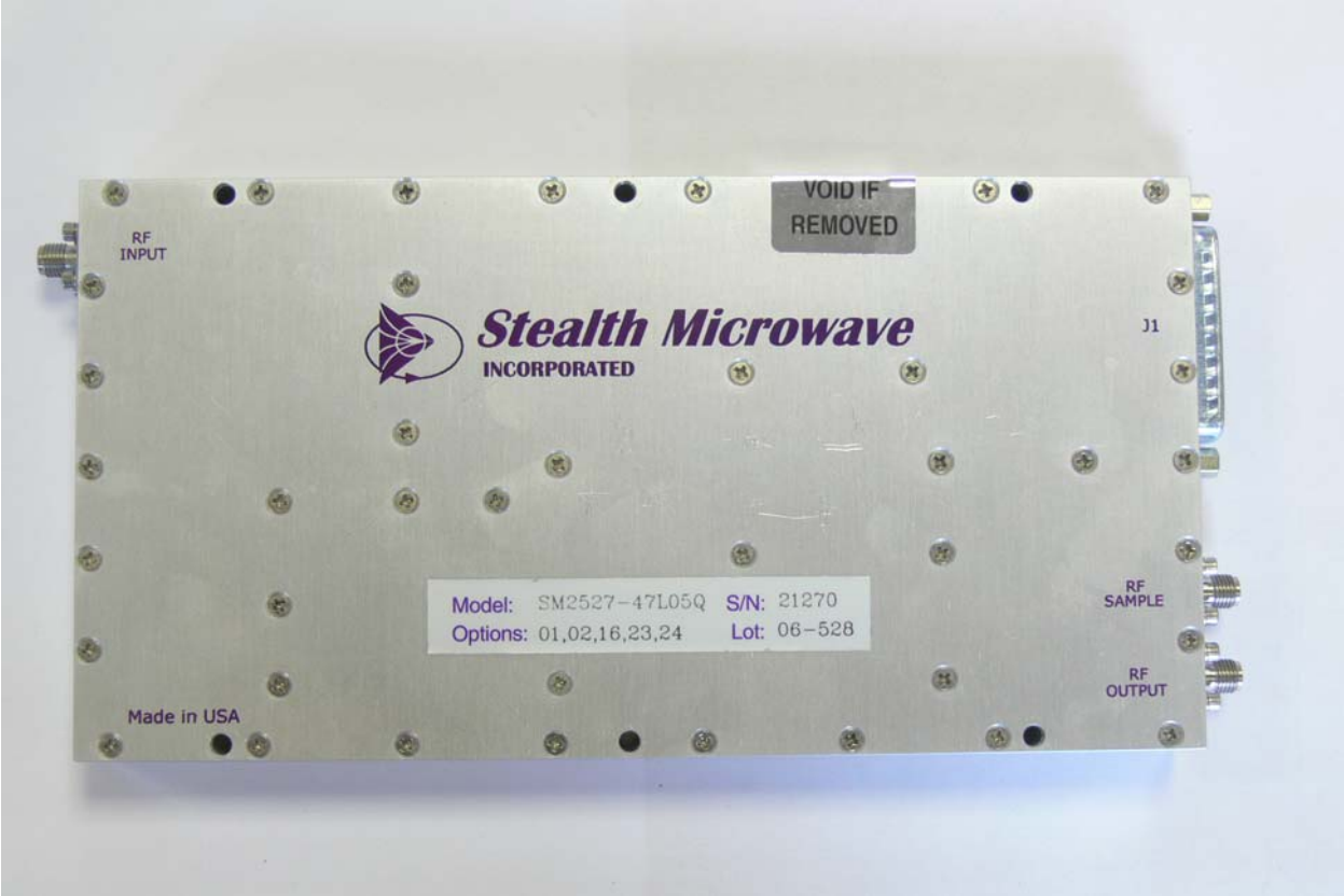
Figure 5: RF Power Amplifier – External
