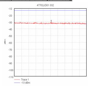
Start 26.5 GHz; Stop 27.0 GHz Ref -10 dBm; Ref Offset -17.7 dB; 10 dB/div RBW 1.0 MHz; VBW 1.0 MHz; Att 20 dB; Swp 50.0 mS Peak 26.755833 GHz, -29.5 dBm Display Line: -13 dBm; Transducer Factors: 26,5-40G 17/10/2005 14:57:30
