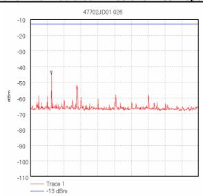
Start 4.0 GHz; Stop 6.0 GHz Ref -10 dBm; Ref Offset 11.8 dB; 10 dB/div RBW 1.0 MHz; VBW 1.0 MHz; Att 0 dB; Swp 50.0 mS Peak 4.25 GHz, -44.83 dBm Display Line: -13 dBm; Transducer Factors: 4G-6G\_Horn(@1m,3m\_cable,A1534) 17/10/2005 14:11:05
