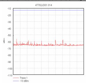
Start 4.0 GHz; Stop 6.0 GHz Ref -10 dBm; Ref Offset 11.8 dB; 10 dB/div RBW 1.0 MHz; VBW 1.0 MHz; Att 10 dB; Swp 50.0 mS Peak 4.0 GHz; -52.83 dBm Display Line: -13 dBm; Transducer Factors: 4G-6G\_Horn(@1m,3m\_cable,A1534) 17/10/2005 12:14:09
