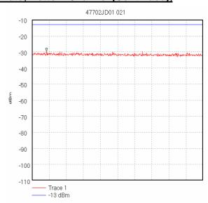
Start 26.5 GHz; Stop 27.0 GHz Ref -10 dBm; Ref Offset -17.7 dB; 10 dB/div RBW 1.0 MHz; VBW 1.0 MHz; Att 20 dB; Swp 50.0 mS Peak 26.5425 GHz, -29.67 dBm Display Line: -13 dBm; Transducer Factors: 26,5-40G 17/10/2005 13:47:31
