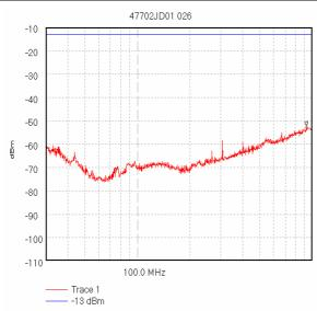
Start 30.0 MHz; Stop 1.0 GHz - Log Scale Ref -10 dBm; Ref Offset 11.8 dB; 10 dB/div RBW 120.0 kHz; VBW 300.0 kHz; Att 0 dB; Swp 80.0 mS Peak 921.438272 MHz, -52.35 dBm Display Line: -13 dBm; ; Limit Test Passed Transducer Factors: A490 10/11/2005 2:39:37 PM
