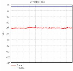
Start 2.0 GHz; Stop 2.5 GHz Ref -10 dBm; Ref Offset 11.8 dB; 10 dB/div RBW 1000.0 kHz; VBW 1.0 MHz; Att 0 dB; Swp 20.0 mS Peak 2.201667 GHz, -47.48 dBm Display Line: -13 dBm; ; Limit Test Passed Transducer Factors: 2 to 4 10/11/2005 10:44:37 AM
