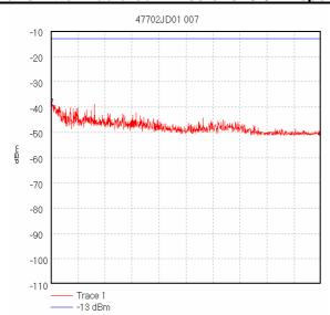
Start 2.686 GHz; Stop 2.69 GHz Ref -10 dBm; Ref Offset 11.8 dB; 10 dB/div RBW 1000.0 kHz; VBW 1.0 MHz; Att 0 dB; Swp 20.0 mS Peak 2.686009 GHz, -38.72 dBm Display Line; -13 dBm; ; Limit Test Passed
