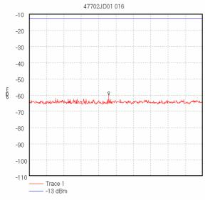
Start 6.0 GHz; Stop 8.0 GHz Ref -10 dBm; Ref Offset 11.8 dB; 10 dB/div RBW 1.0 MHz; VBW 1.0 MHz; Att 0 dB; Swp 50.0 mS Peak 6.916667 GHz, -60.0 dBm Display Line: -13 dBm; Transducer Factors: 6G-8G\_Horn(@1m,3m\_cable,A1534) 17/10/2005 12:27:52
