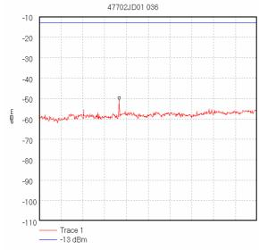
Start 8.0 GHz; Stop 12.5 GHz Ref -10 dBm; Ref Offset 11.8 dB; 10 dB/div RBW 1.0 MHz; VBW 1.0 MHz; Att 0 dB; Swp 90.0 mS Peak 9.65 GHz, -51.17 dBm Display Line: -13 dBm; Transducer Factors: 8G-12,6G\_Horn(@1m,3m\_cable,A1534) 17/10/2006 15:17:27
