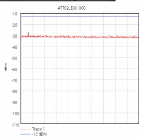
Start 26.5 GHz; Stop 27.0 GHz Ref -10 dBm; Ref Offset -17.0 dB; 10 dB/div RBW 1.0 MHz; VBW 1.0 MHz; Att 20 dB; Swp 50.0 mS Peak 26.5325 GHz, -29.67 dBm Display Line: -13 dBm; Transducer Factors: 26,5-40G 17/10/2005 11:46:56
