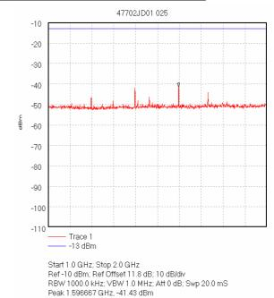
Display Line: -13 dBm; ; Limit Test Passed Transducer Factors: 1 to 2
