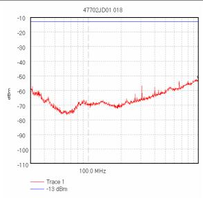
Start 30.0 MHz; Stop 1.0 GHz - Log Scale Ref -10 dBm; Ref Offset 11.8 dB; 10 dB/div RBW 120.0 kHz; VBW 300.0 kHz; Att 0 dB; Swp 380.0 mS Peak 988.379648 MHz, -52.15 dBm Display Line: -13 dBm; Limit Test Passed Transducer Factors; A490 10/11/2005 12:22:06 PM
