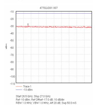
Peak 26,579167 GHz, -29.5 dBm Display Line: -13 dBm; Transducer Factors: 26,5-40G 17/10/2005 11:45:45
