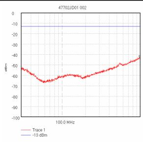
Start 30.0 MHz; Stop 1.0 GHz - Log Scale Ref 0 dBm; Ref Offset 11.8 dB; 10 dB/div RBW 120.0 kHz; VBW 300.0 kHz; Att 0 dB; Swp 80.0 mS Peak 973.09548 MHz, -42.99 dBm Limit/Mask; ; Limit Test Passed Transducer Factors: A490 10/11/2005 10:23:55 AM
