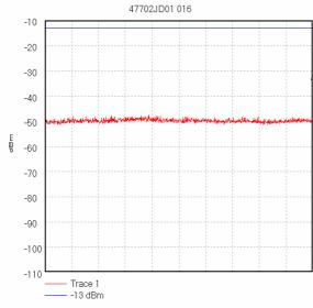
Start 2.0 GHz; Stop 2.5 GHz Ref -10 dBm; Ref Offset 11.8 dB; 10 dB/div RBW 1000.0 kHz; VBW 1.0 MHz; Att 0 dB; Swp 20.0 mS Peak 2.5 GHz, -35.06 dBm Display Line: -13 dBm; ; Limit Test Passed Transducer Factors: 2 to 4 10/11/2005 12:04:28 PM
