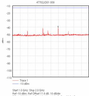
Start 1.0 GHz; Stop 2.0 GHz Ref -10 dBm; Ref Offset 11.8 dB; 10 dB/div RBW 1000.0 kHz; VBW 1.0 MHz; Att 0 dB; Swp 20.0 mS Peak 1.596667 GHz, -40.65 dBm Display Line: -13 dBm; ; Limit Test Passed Transducer Factors: 1 to 2 10/11/2005 11:12:11 AM
