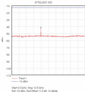
Start 8.0 GHz; Stop 12.5 GHz Ref -10 dBm; Ref Offset 11.8 dB; 10 dB/div RBW 1.0 MHz; VBW 1.0 MHz; Att 10 dB; Swp 90.0 mS Peak 9.785 GHz, -42.67 dBm Display Line: -13 dBm; Transducer Factors: 12.5-18G\_Horn(@1m.3m\_cable,A1534) 17/10/2005 10:53:30
