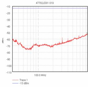
Start 30.0 MHz; Stop 1.0 GHz - Log Scale Ref -10 dBm; Ref Offset 11.8 dB; 10 dB/div RBW 120.0 kHz; VBW 300.0 kHz; Att 0 dB; Swp 80.0 mS Peak 976.894208 MHz, -52.2 dBm Display Line: -13 dBm; ; Limit Test Passed Transducer Factors: A490
