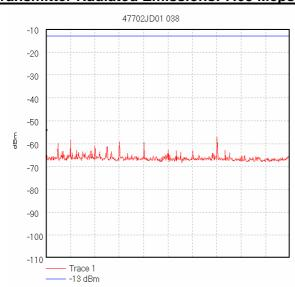
Start 4.0 GHz; Stop 6.0 GHz Ref -10 dBm; Ref Offset 11.8 dB; 10 dB/div RBW 1.0 MHz; VBW 1.0 MHz; Att 0 dB; Swp 50.0 mS Peak 4.0 GHz, -55.67 dBm Display Line: -13 dBm; Transducer Factors: 4G-6G\_Horn(@1m,3m\_cable,A1534) 17/10/2005 15:25:04
