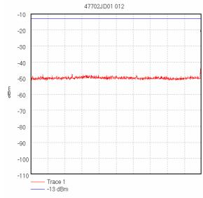
Start 2.0 GHz; Stop 2.5 GHz Ref -10 dBm; Ref Offset 11.8 dB; 10 dB/div RBW 1000.0 kHz; VBW 1.0 MHz; Att 0 dB; Swp 20.0 mS Peak 2.5 GHz, -22.49 dBm Display Line: -13 dBm; ; Limit Test Passed Transducer Factors: 2 to 4 10/11/2005 11:32:49 AM
