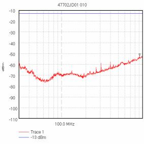
Start 30.0 MHz; Stop 1.0 GHz - Log Scale Ref -10 dBm; Ref Offset 11.8 dB; 10 dB/div RBW 120.0 kHz; VBW 300.0 kHz; Att 0 dB; Swp 80.0 mS Peak 910.730752 MHz, -52.0 dBm Display Line: -13 dBm; ; Limit Test Passed Transducer Factors: A490
