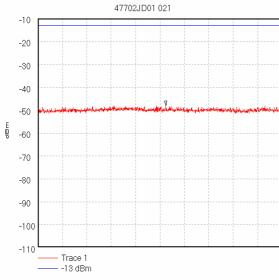
Start 2.0 GHz; Stop 2.5 GHz Ref -10 dBm; Ref Offset 11.8 dB; 10 dB/div RBW 1000.0 kHz; VBW 1.0 MHz; Att 0 dB; Swp 20.0 mS Peak 2.26222 GHz, -47.83 dBm Display Line: -13 dBm; ; Limit Test Passed Transducer Factors: 2 to 4 10/11/2005 2:04:32 PM
