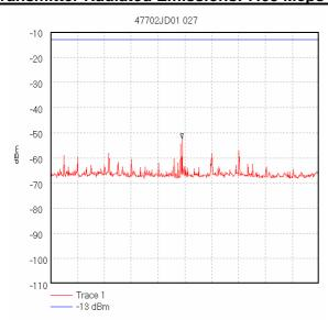
Start 4.0 GHz; Stop 6.0 GHz Ref -10 dBm; Ref Offset 11.8 dB; 10 dB/div RBW 1.0 MHz; VBW 1.0 MHz; Att 0 dB; Swp 50.0 mS Peak 4.98 GHz, -52.17 dBm Display Line: -13 dBm; Transducer Factors: 4G-6G\_Horn(@1m,3m\_cable,A1534) 17/10/2005 14:38:14
