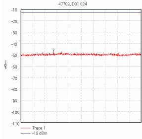
Start 2.0 GHz; Stop 2.5 GHz Ref -10 dBm; Ref Offset 11.8 dB; 10 dB/div RBW 1000.0 kHz; VBW 1.0 MHz; Att 0 dB; Swp 20.0 mS Peak 2.136111 GHz, -46.69 dBm Display Line: -13 dBm; ; Limit Test Passed Transducer Factors: 2 to 4 10/11/2005 2:24:52 PM
