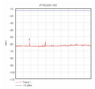
Start 6.0 GHz; Stop 8.0 GHz Ref-10 dBm; Ref Offset 11.8 dB; 10 dB/div RBW 1.0 MHz; VBW 1.0 MHz; Att 10 dB; Swp 50.0 mS Peak 6.366667 GHz, -54.83 dBm Display Line: -13 dBm; Transducer Factors: 6G-8G\_Horn(@1m,3m\_cable,A1534) 17/10/2005 10:27:17
