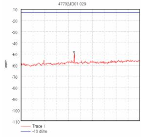
Start 8.0 GHz; Stop 12.5 GHz Ref -10 dBm; Ref Offset 11.8 dB; 10 dB/div RBW 1.0 MHz; VBW 1.0 MHz; Att 0 dB; Swp 90.0 mS Peak 10.01 GHz, -49.67 dBm Display Line; -13 dBm; Transducer Factors: 8G-12,5G\_Horn(@1m,8m\_cable,A1534) 17/10/2006 14 46:44
