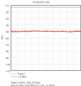
Ref-10 dBm; Ref Offset 11.8 dB; 10 dB/div RBW 1000.0 kHz; VBW 1.0 MHz; Att 0 dB; Swp 20.0 mS Peak 2.0 GHz, -47.68 dBm Display Line: -13 dBm; ; Limit Test Passed Transducer Factors: 2 to 4 10/11/2005 11:07:07 AM
