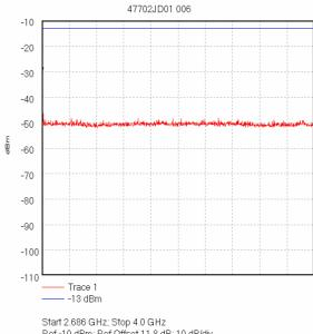
Start 2.686 GHz; Stop 4.0 GHz Ref -10 dBm; Ref Offset 11.8 dB; 10 dB/div RBW 1000.0 kHz; VBW 1.0 MHz; Att 0 dB; Swp 20.0 mS Peak 2.686 GHz, -30.34 dBm Display Line: -13 dBm; ; Limit Test Passed Transducer Factors: 2 to 4 10/11/2005 10:57:27 AM
