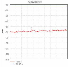
Start 8.0 GHz; Stop 12.5 GHz Ref -10 dBm; Ref Offset 11.8 dB; 10 dB/div RBW 1.0 MHz; VBW 1.0 MHz; Att 0 dB; Swp 90.0 mS Peak 9.71 GHz, -54.17 dBm Display Line: -13 dBm; Transducer Factors: 8G-12,5G\_Horn(@1m,3m\_cable,A1534) 17/10/2006 14:04:07
