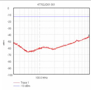
Start 30.0 MHz; Stop 1.0 GHz - Log Scale Ref 0 dBm; Ref Offset 11.8 dB; 10 dB/div RBW 120.0 kHz; VBW 300.0 kHz; Att 0 dB; Swp 380.0 mS Peak 958.047488 MHz; -42.66 dBm Limit/Mask; Limit Test Passed Transducer Factors: A490 10/11/2005 10:11:04 AM
