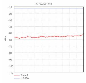
Start 8.0 GHz; Stop 12.5 GHz Ref -10 dBm; Ref Offset 11.8 dB; 10 dB/div RBW 1.0 MHz; VBW 1.0 MHz; Att 10 dB; Swp 90.0 mS Peak 12.4925 GHz, -51.83 dBm Display Line: -13 dBm; Transducer Factors: 8G-12.5G\_Horn(@1m,3m\_cable,A1534) 17/10/2005 12:06:12
