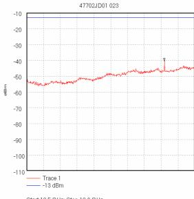
Start 12.5 GHz; Stop 18.0 GHz Ref-10 dBm; Ref Offset 11.8 dB; 10 dB/div RBW 1.0 MHz; VBW 1.0 MHz; Att 0 dB; Swp 110.0 mS Peak 17.01 GHz, -40.5 dBm Display Line: -13 dBm; Transducer Factors: 12.5-18G\_Horn(@1m,3m\_cable,A1534) 17/10/2005 13:59:40
