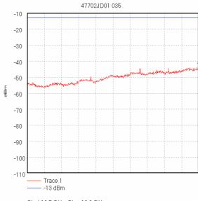
Start 12.5 GHz; Stop 18.0 GHz Ref -10 dBm; Ref Offset 11.8 dB; 10 dB/div RBW 1.0 MHz; VBW 1.0 MHz; Att 0 dB; Swp 110.0 mS Peak 18.0 GHz, -43.0 dBm Display Line: -13 dBm; Transducer Factors: 12.5-18G\_Horn(@1m,3m\_cable,A1534) 17/10/2005 15:13:38
