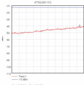
Start 12.5 GHz; Stop 18.0 GHz Ref -10 dBm; Ref Offset 11.8 dB; 10 dB/div RBW 1.0 MHz; VBW 1.0 MHz; Att 10 dB; Swp 110.0 mS Peak 17.679167 GHz, -40.67 dBm Display Line: -13 dBm; Transducer Factors: 12.5-18G\_Horn(@1m,3m\_cable,A1534) 17/10/2005 12:08:53
