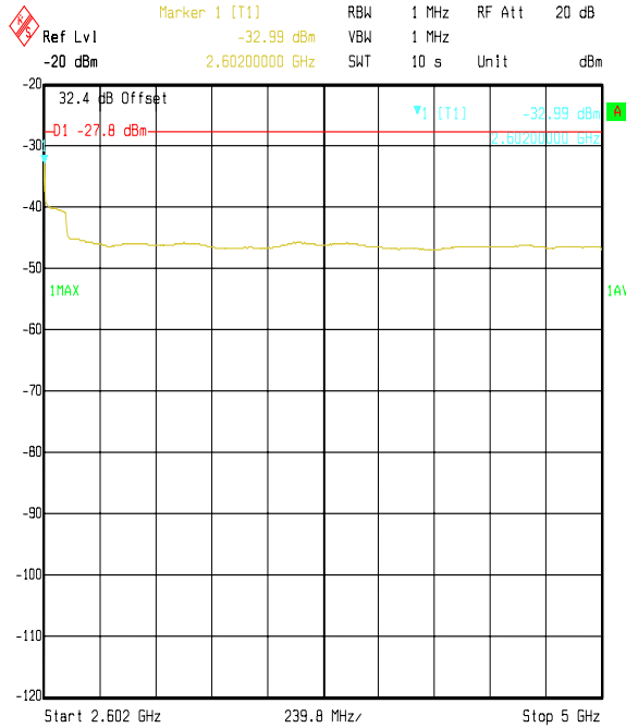
Title: IPWireless EUT: 2.5GHz DN/DZ FCC P15/21/74. Cond. Spurious Comment A: 45361JD05 Middle Channel 3.84 Mcps 2.602-5 GHz Avg Detector Date: 10.FEB.2004 14:57:45
