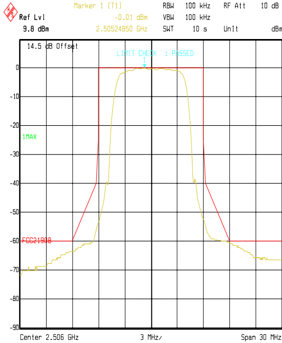
Title: IPWireless EUT: 2.5GHz DN/DZ FCC P15/21/74. Spectrum Mask Comment A: 45361JD05 Bottom Channel 7.68 Mcps Date: 10.FEB.2004 12:20:12
