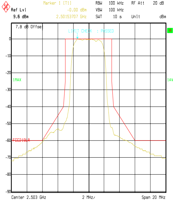
Title: IPWireless EUT: 2.5GHz DN/DZ FCC P15/21/74. Spectrum Mask Comment A: 45361JD05 Bottom Channel 3.84 Mcps Date: 10.FEB.2004 12:22:58
