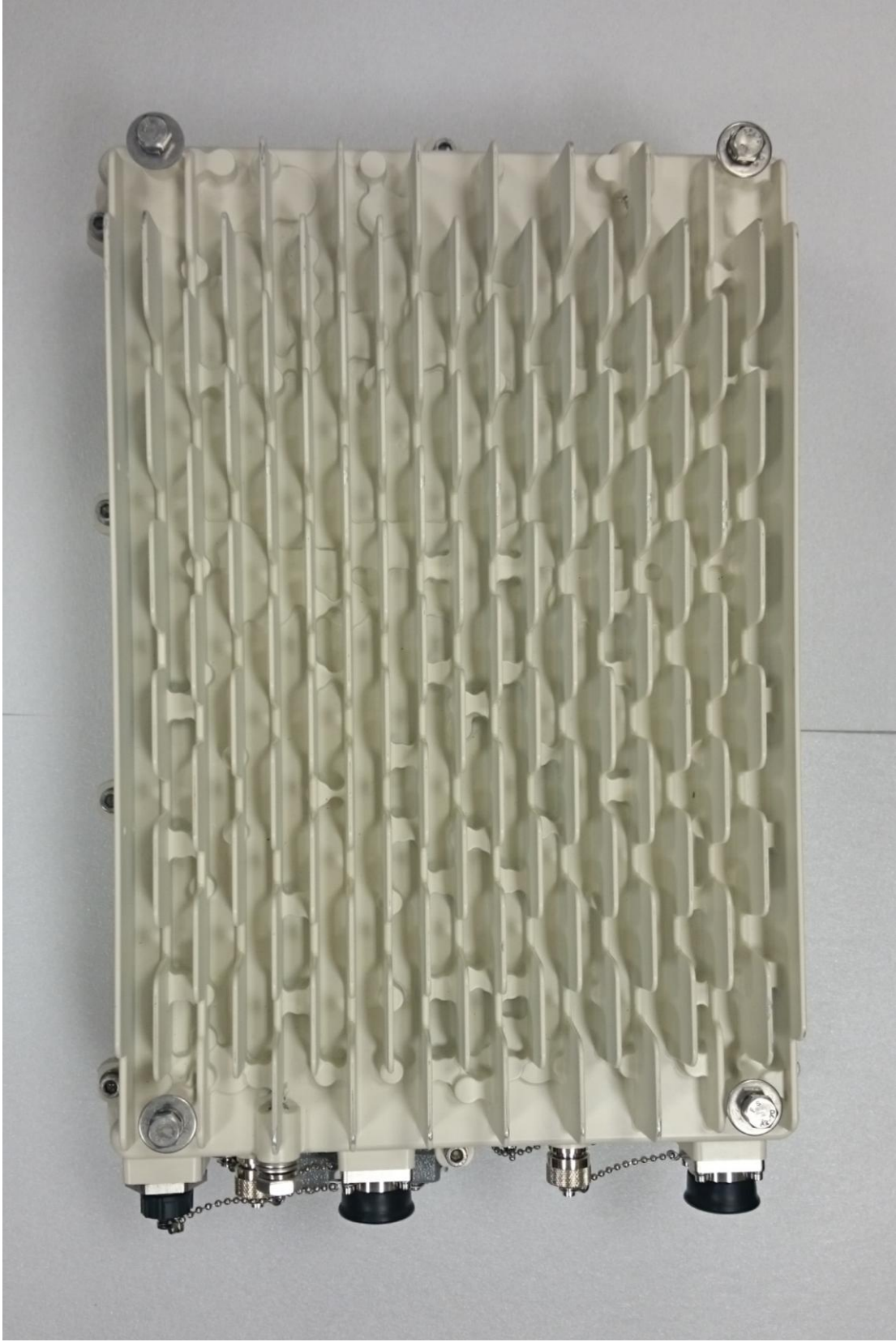
Figure 2: RN2420 eNodeB Rear View
