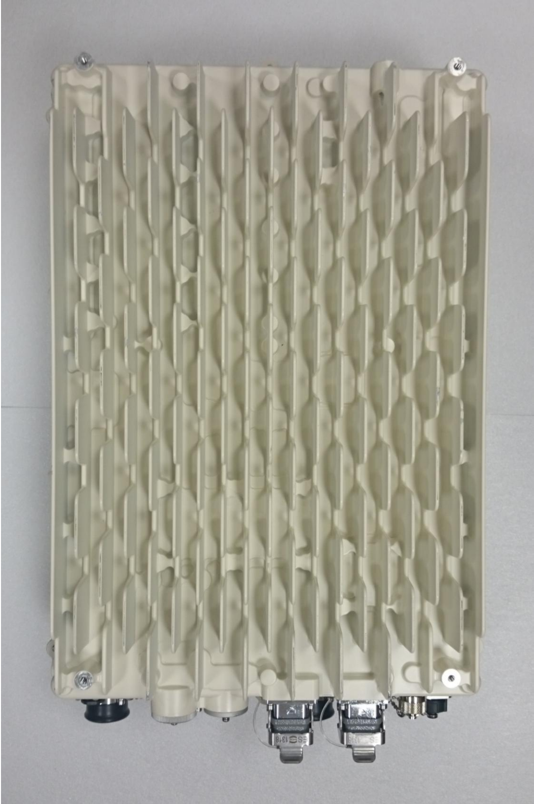
Figure 1: RN2420 eNodeB Front View
