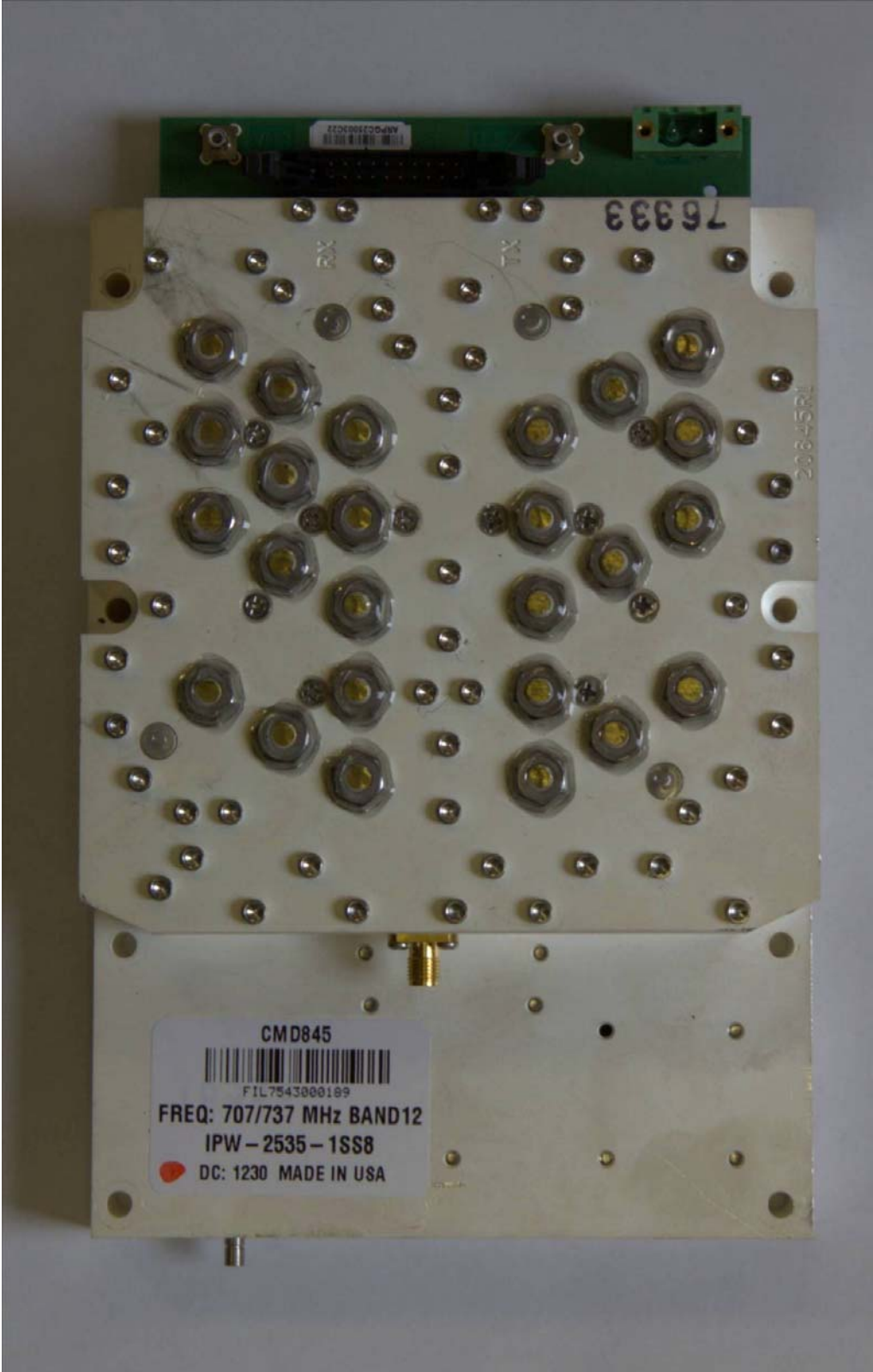
Figure 5: Power Amplifier and Filter Assembly Top View
