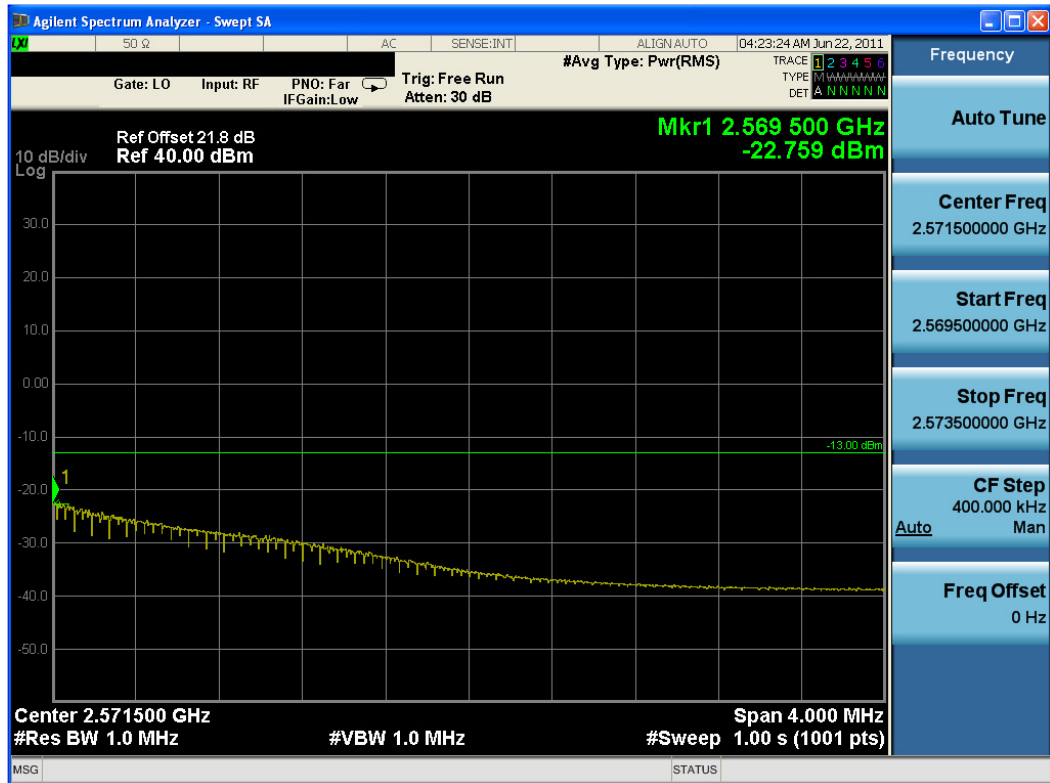
Plot 7-20. Hi 4MHz Plot (TD-CDMA 64-QAM) Antenna Port 1
