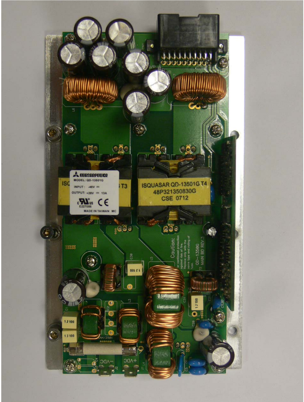
Figure 5: 28VDC Power Supply
