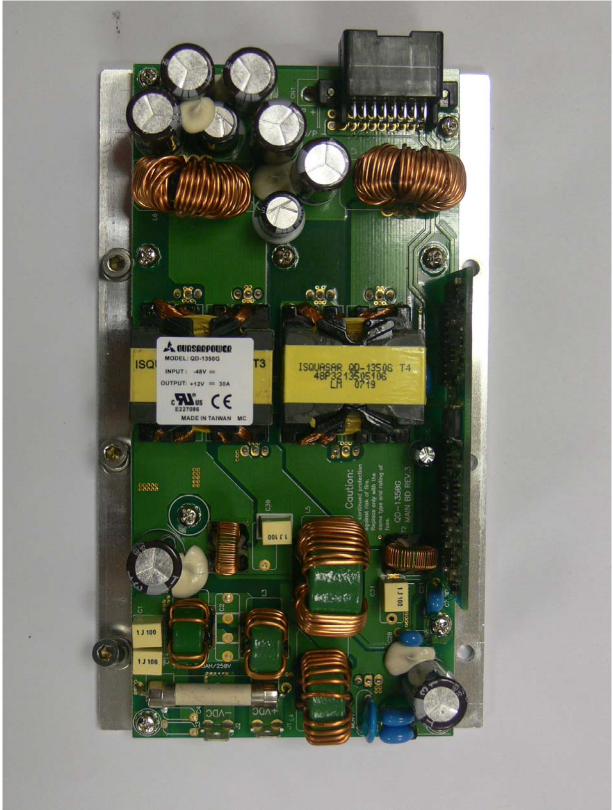
Figure 6: 12VDC Power Supply
