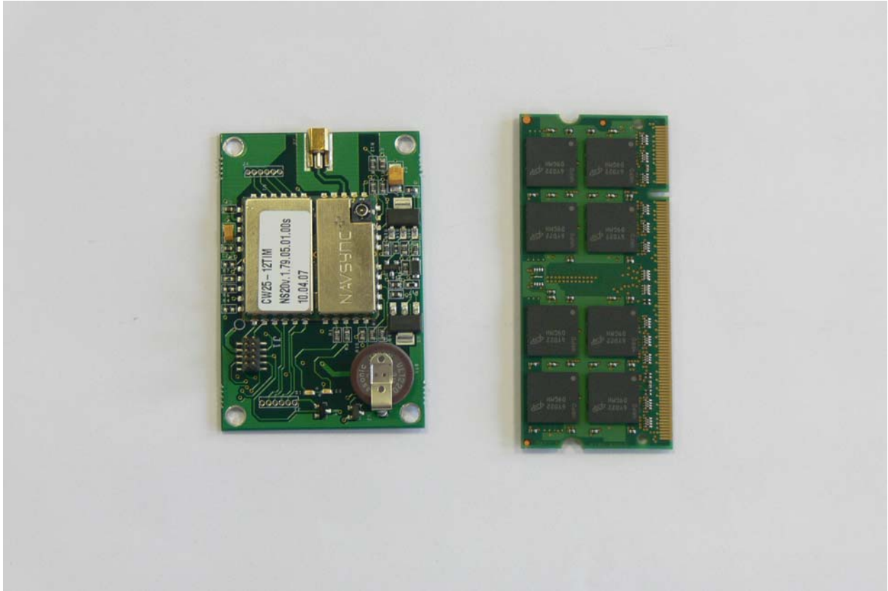
Figure 7: GPS & Memory Modules - Bottom
