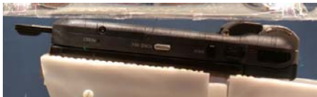
Figure 8-2 CompactFlash radio card in PDA host configuration
