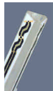
Figure 3.2 Probe Thick-Film Technique
