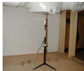
Figure 12.1 Dipole Validation Test Setup
