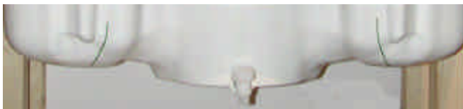
Figure 7.2 SAM Twin Phantom shell
