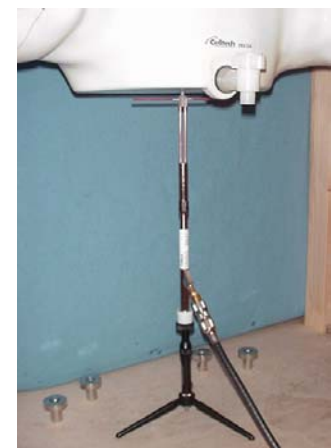
835 MHz Dipole Setup
