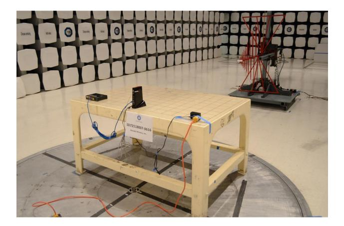
Radiated Emissions Test Setup (below 1GHz Back)
