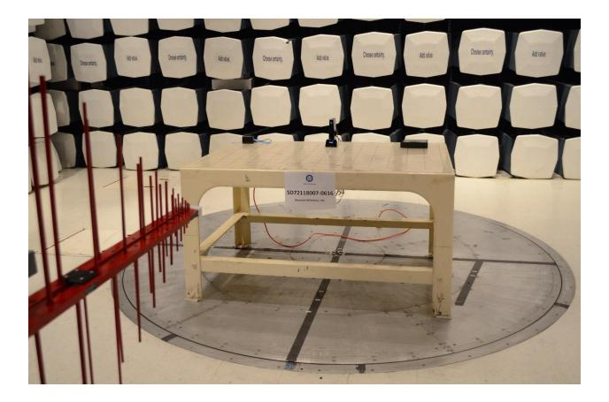
Radiated Emissions Test Setup (below 1GHz Front)
