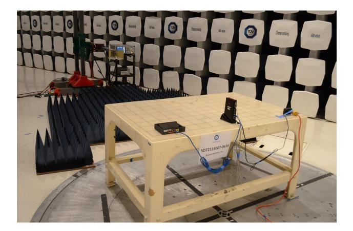
Radiated Emissions Test Setup (above 1GHz Back)
