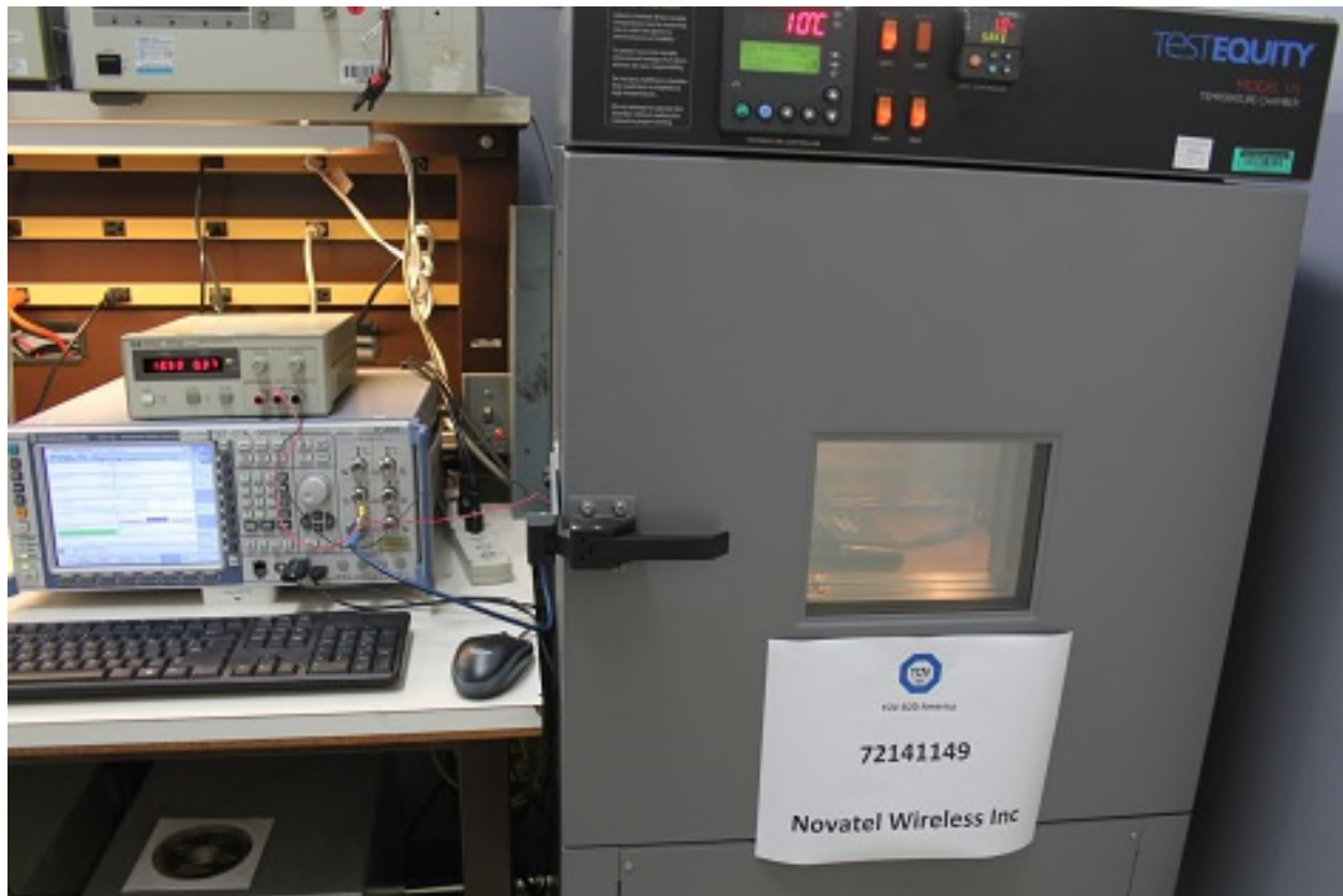
Frequency Stability Test Setup
