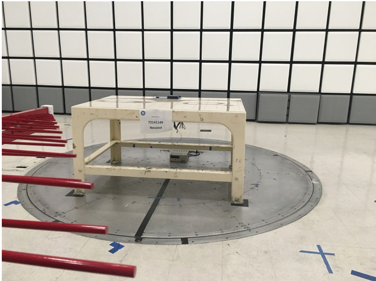
FCC Part 15B Radiated Emissions Test Setup (below 1GHz)
