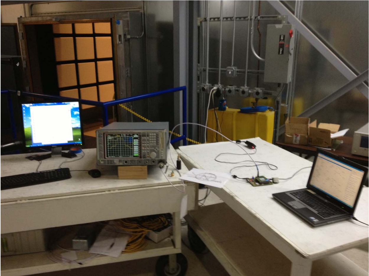
Band edge and occupied bandwidth test setup
