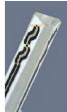
Figure 2.3 Probe Thick-Film Technique
