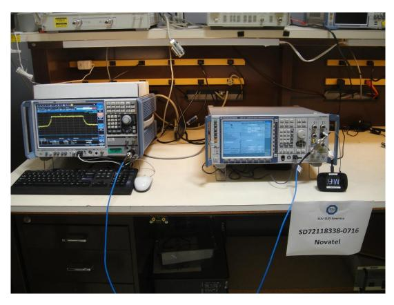
**Antenna Conducted Port Bench Measurement**
