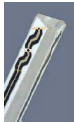
Figure 2.3 Probe Thick-Film Technique
