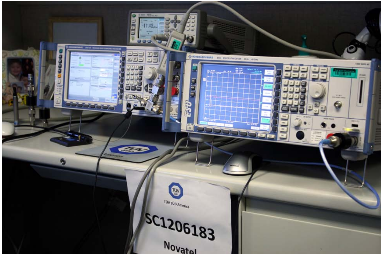
Conducted Port Measurement (GSM,WCDMA and LTE)
