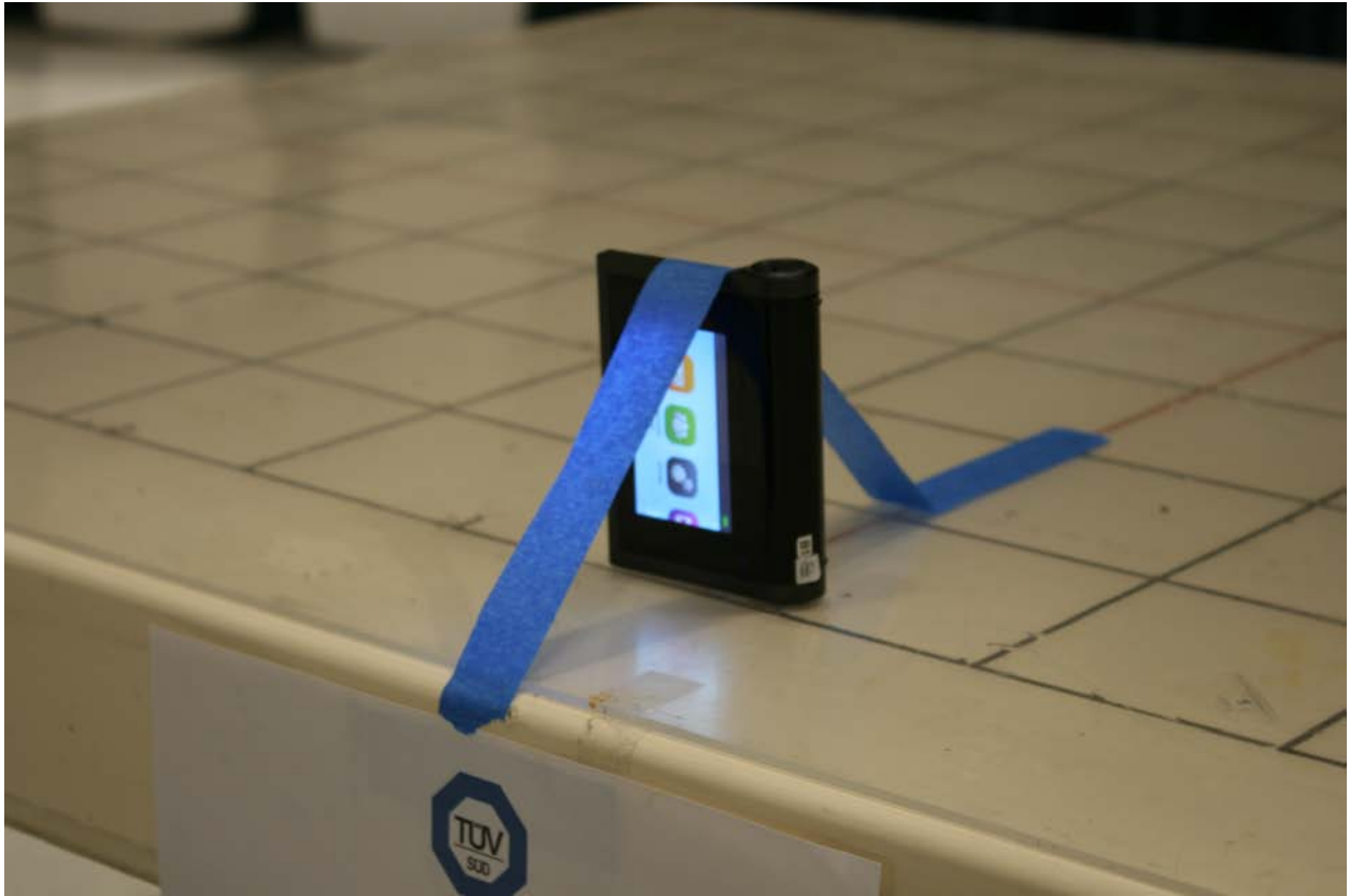
Radiated Emission Test Setup (Y Configuration)
