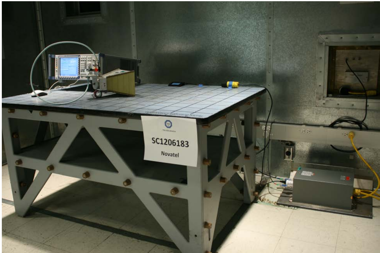
Conducted Emission Test Setup (GSM,WCDMA and LTE)
