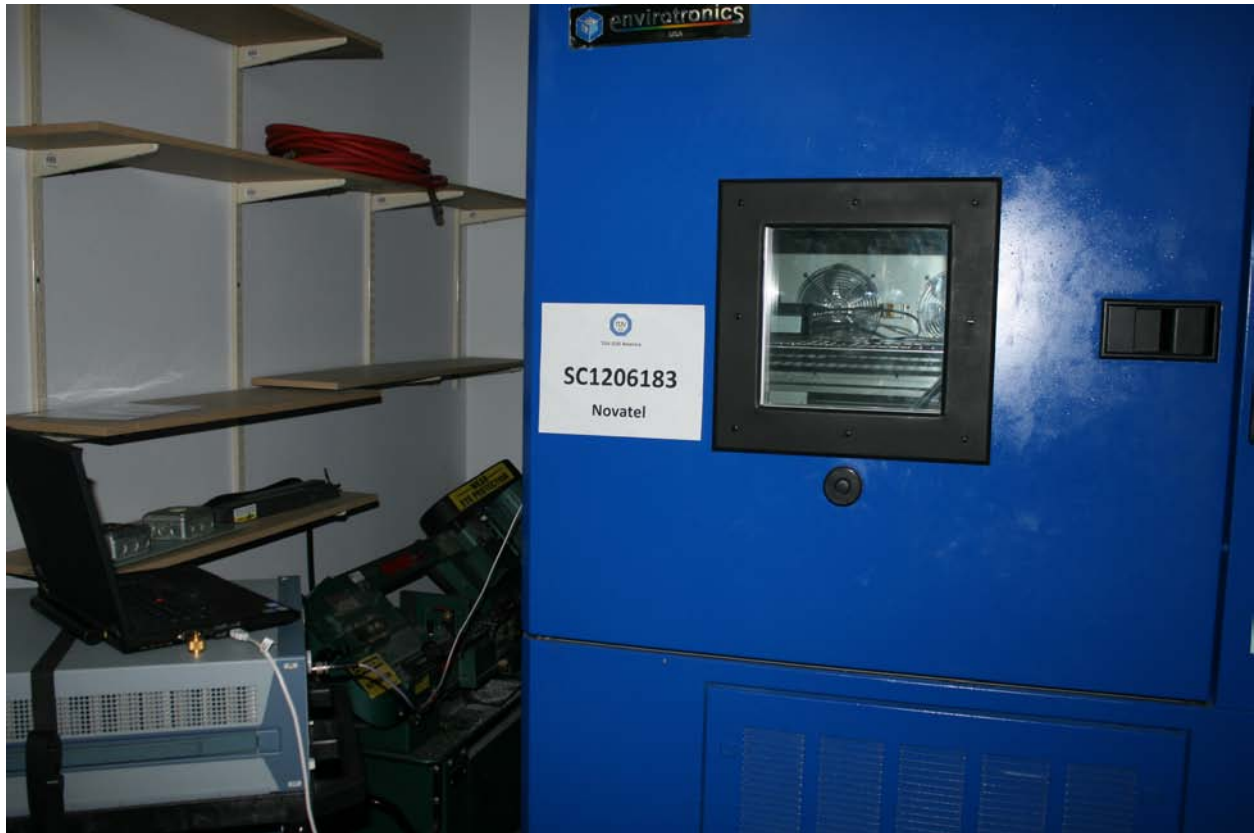
Frequency Stability (FCC Part 22,24 and 27)
