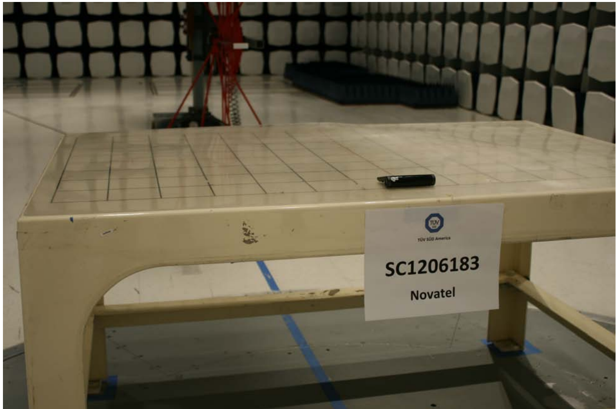
Radiated Emission Test Setup (below 1GHz FCC Part 15 Subpart C)
