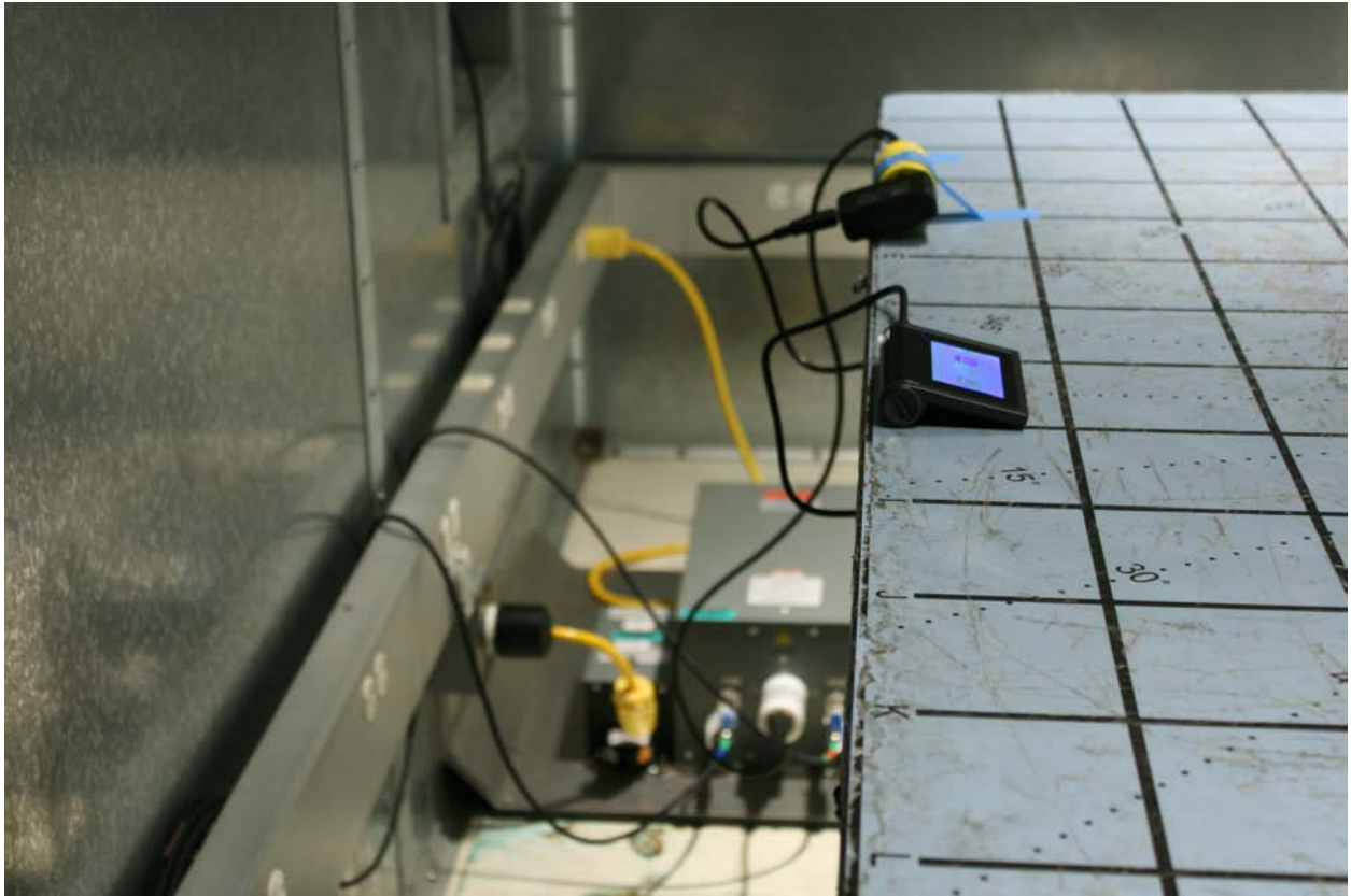
Conducted Emission Test Setup (WiFi)
