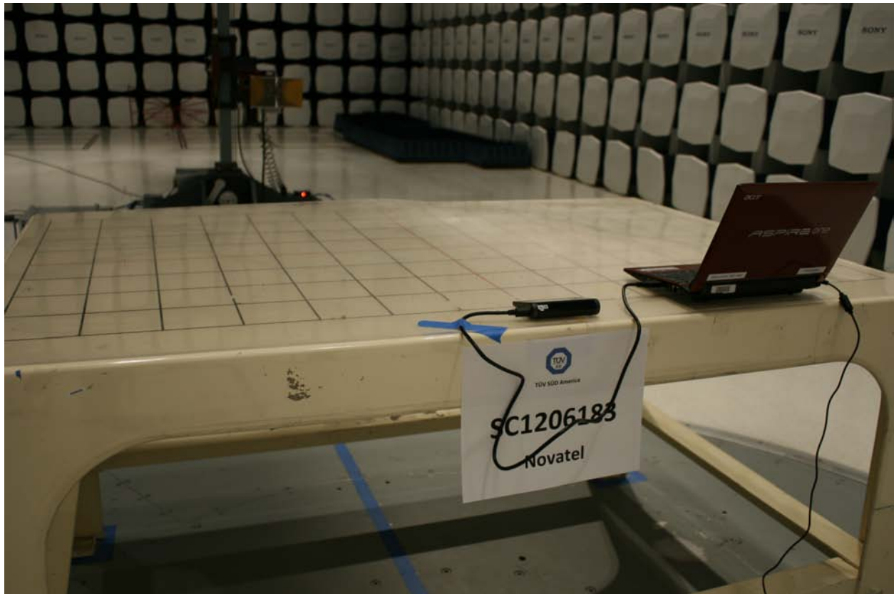
Radiated Emission Test Setup (above 1GHz FCC Part 15 Subpart B)
