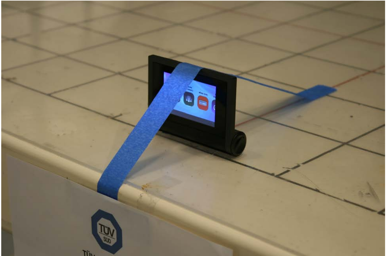
Radiated Emission Test Setup (X Configuration)
