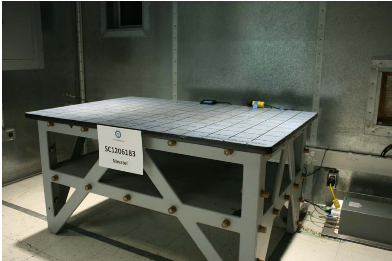
Conducted Emission Test Setup (WiFi)
