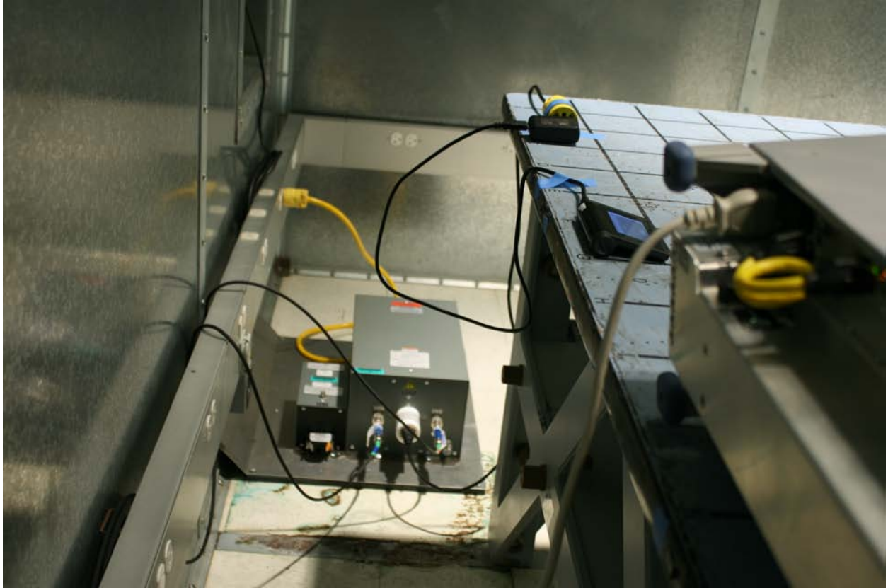
Conducted Emission Test Setup (GSM,WCDMA and LTE)
