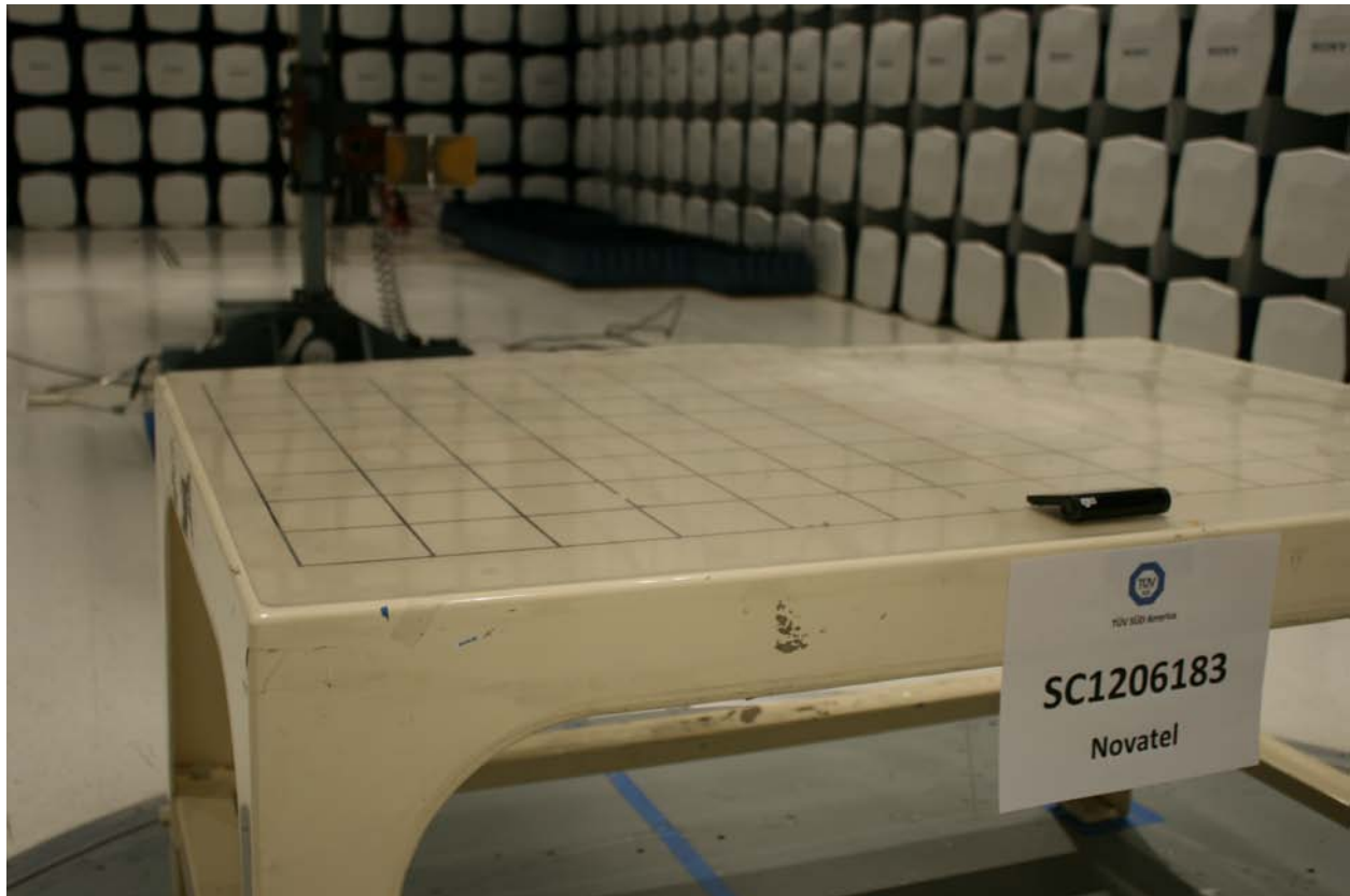
Radiated Emission Test Setup (above 1GHz FCC Part 15 Subpart C)
