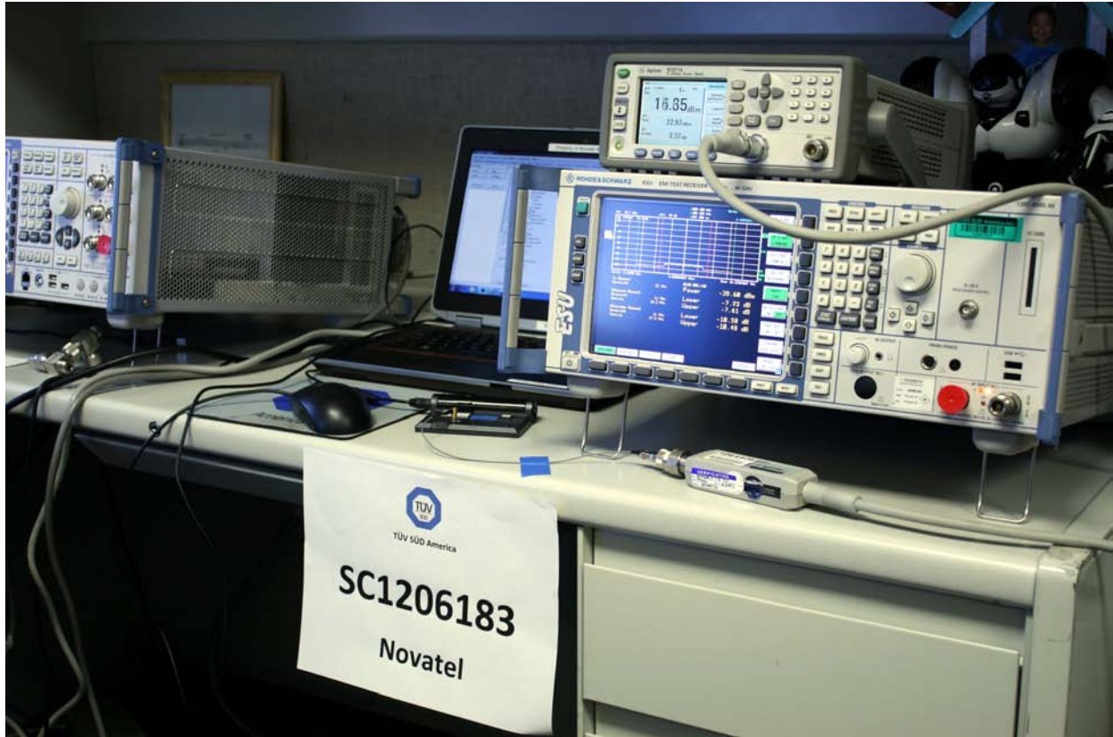
Conducted Port Measurement using power meter (WiFi)
