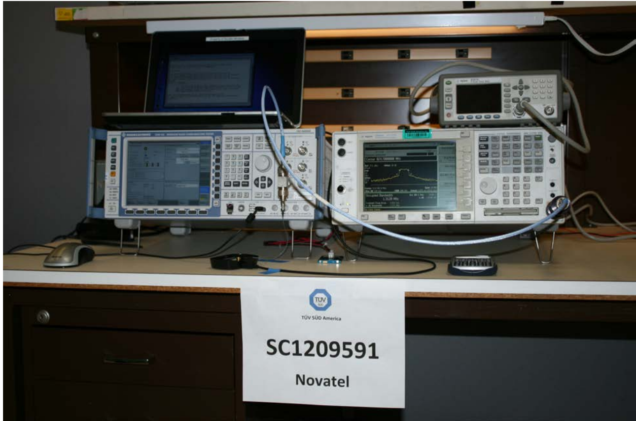
Conducted Port Measurement (CDMA and LTE)
