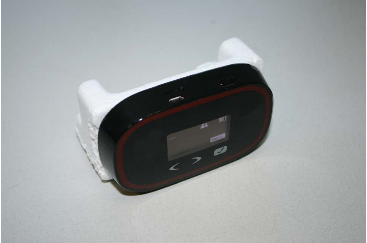
Radiated Emission Test Setup (Y Configuration)
