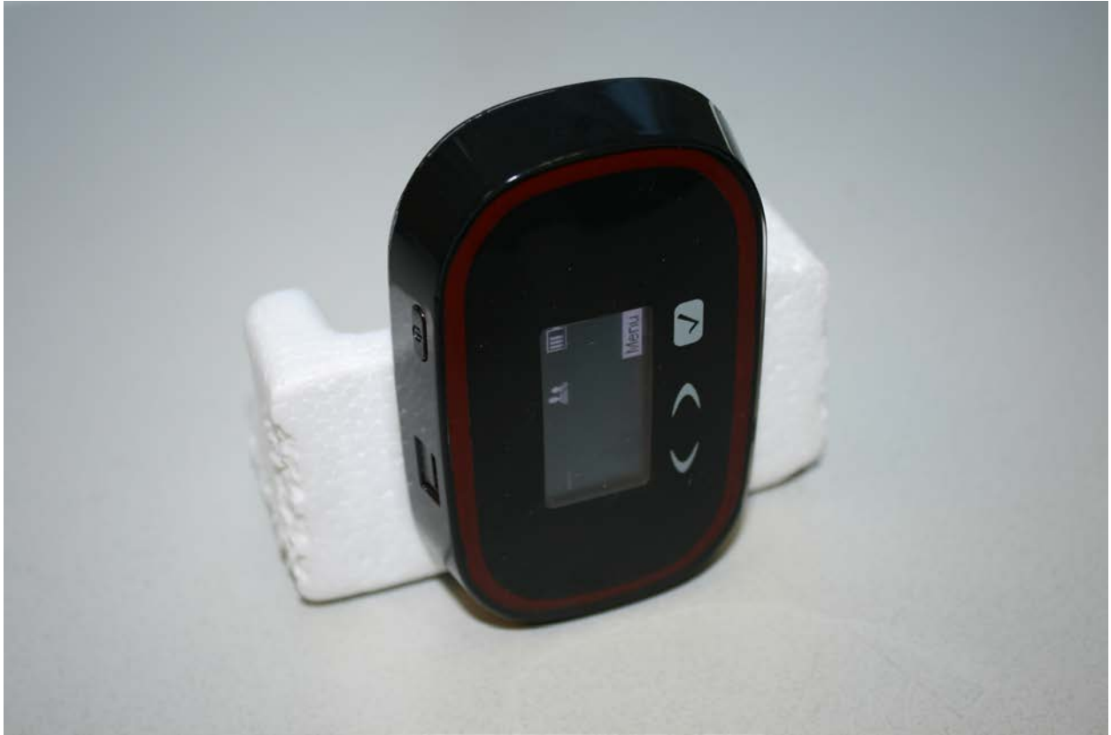
Radiated Emission Test Setup (Z Configuration)
