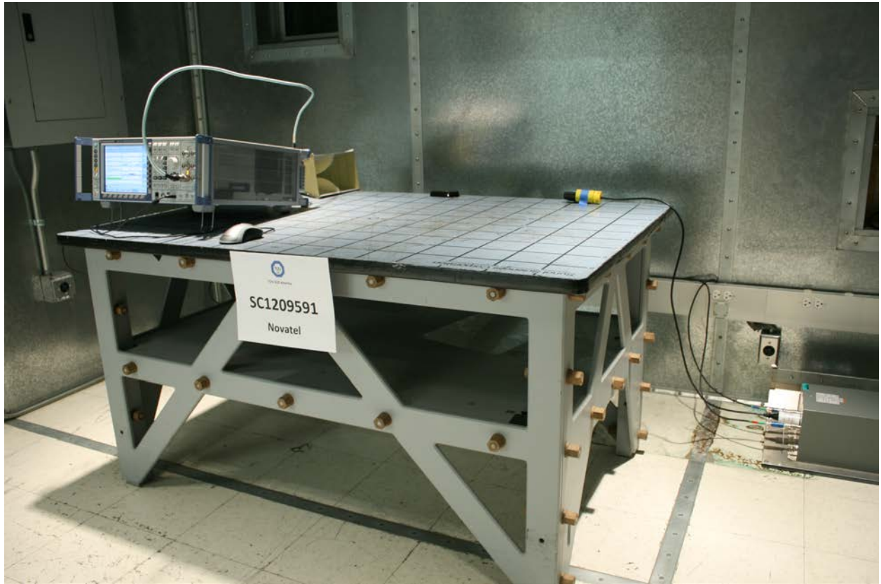
Conducted Emission Test Setup (CDMA and LTE)
