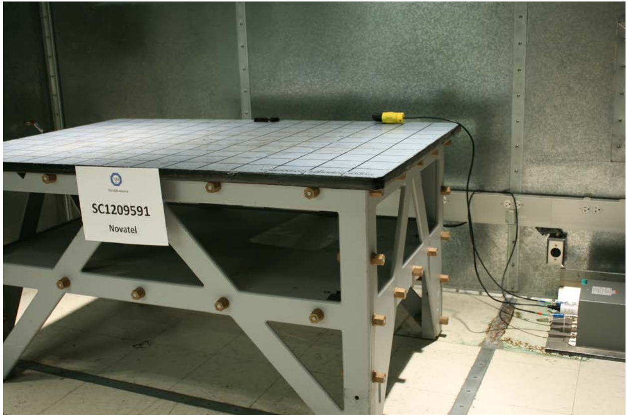
Conducted Emission Test Setup (WiFi)
