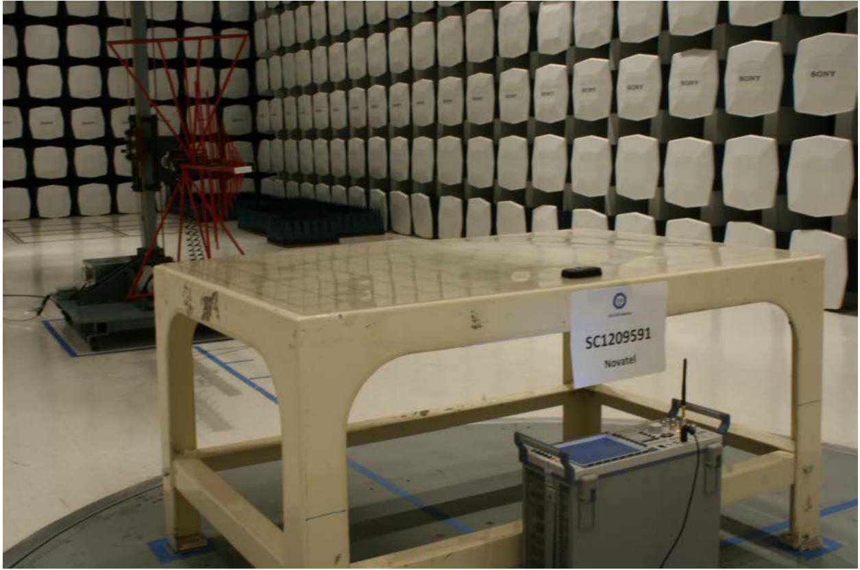
Radiated Emission Test Setup (below 1GHz FCC Part 22,24 and 27)
