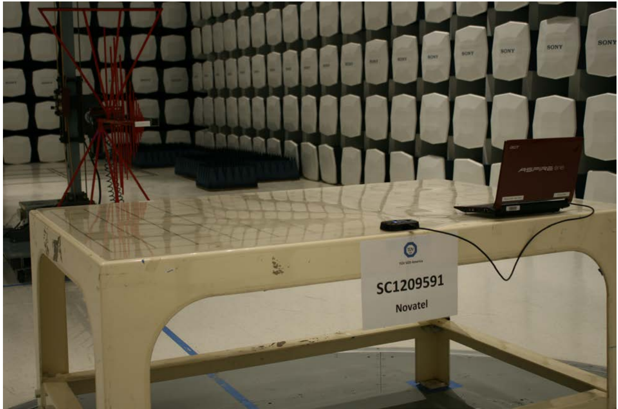
Radiated Emission Test Setup (below 1GHz FCC Part 15 Subpart B)
