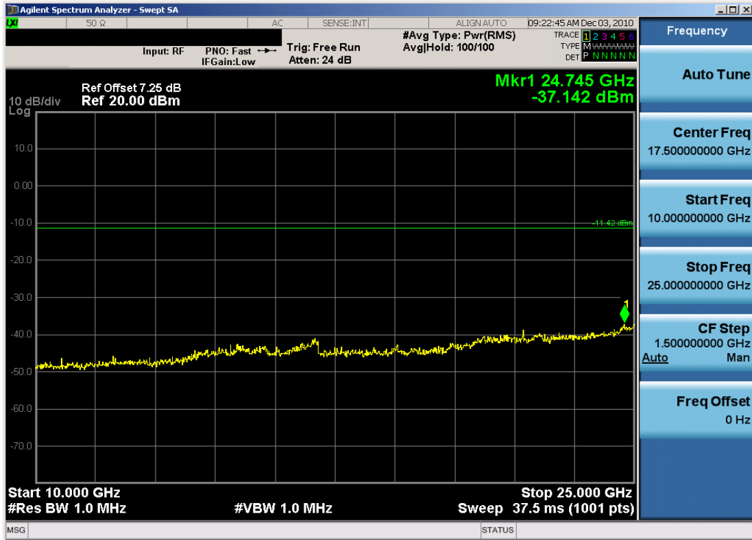
Plot 6-30. Conducted Spurious Plot (802.11b – Ch. 11)
