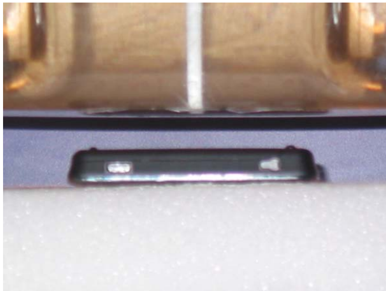
Bottom Face Test Position 12 mm Gap
