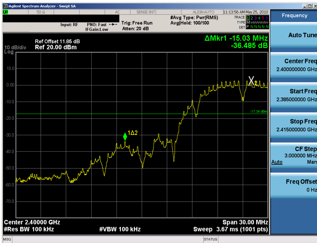
Plot 6-7. Band Edge Plot (802.11b – Ch. 1)
